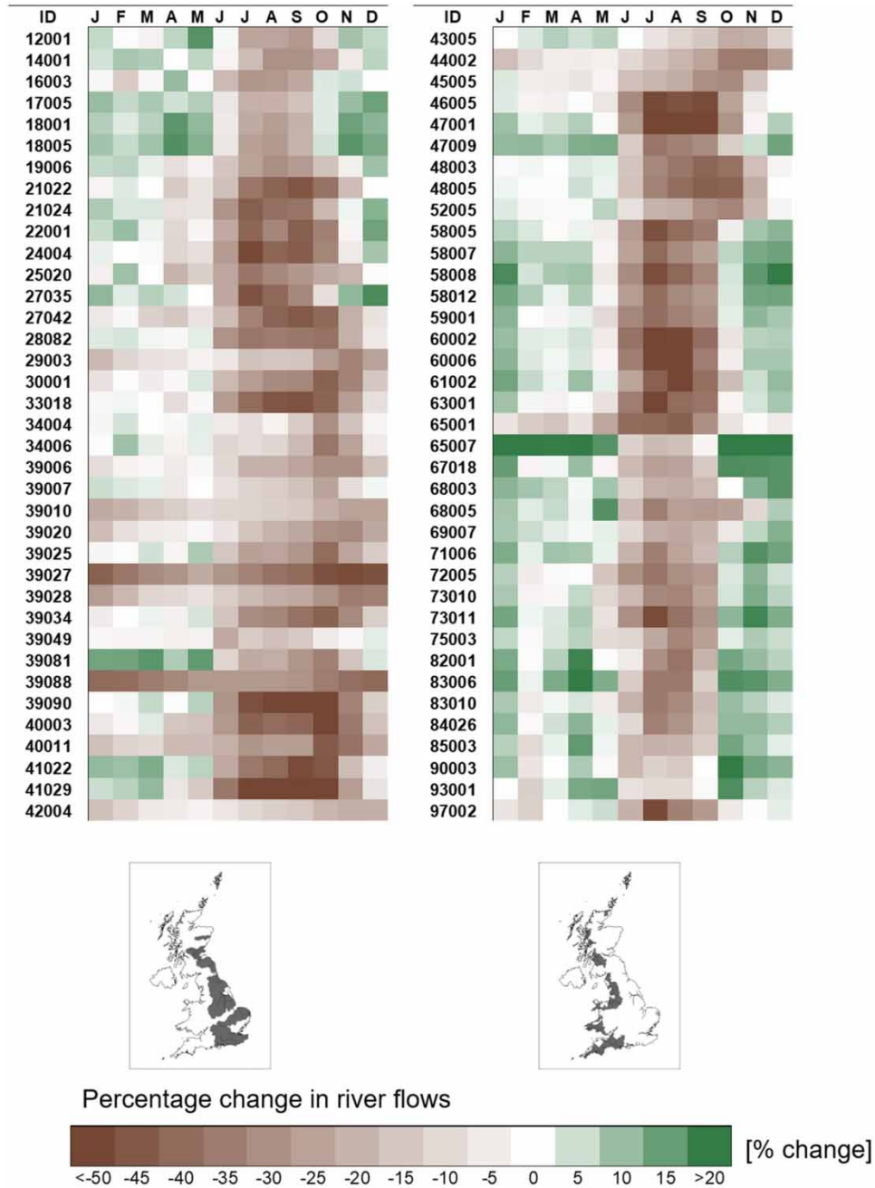
Figure 3 | Monthly percentage changes in river flows at the gauging station near RoR schemes. The baseline flows are the flows simulated using the GR6J hydrological model for the period 1980–2009. The near future flows are the mean for all the regional climate models (RCMs) simulated flows for the period 2030–2059. The maps below show the highlighted in grey the catchments where the gauges are in each column. Furthermore, the ID is equivalent to the gauge number, which is based on the NRFA system, consisting of the hydrometric area number, followed by three further digits (e.g., the IDs 21022 and 21024 correspond to hydrometric area 21, also known as the Tweed catchment). The legend refers to percentage change in mean monthly flows in the future from the baseline.
