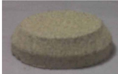
Figure 2 | Nano-silver treated porous disc.
