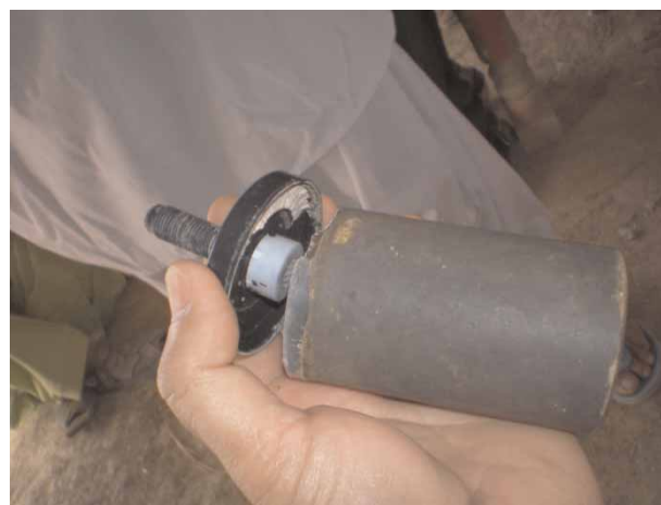
Figure 3 | Broken ceramic filter.
