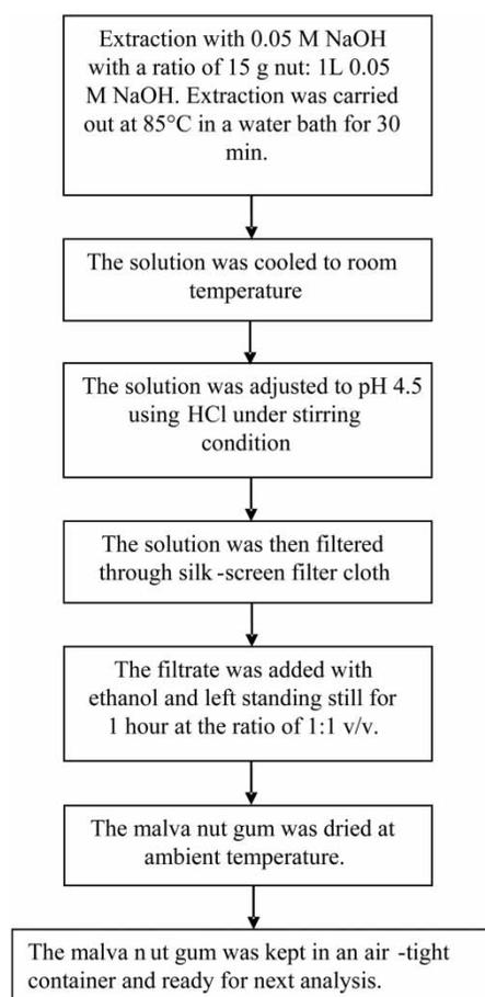
Figure 1 | Schematic diagram of MNG extraction process.
