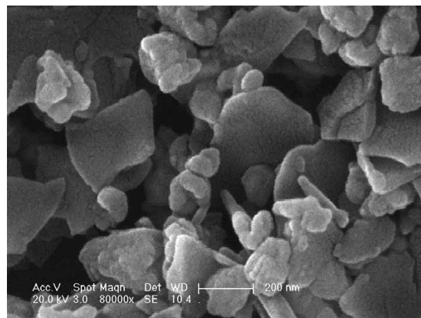
Figure 1 | SEM photograph of ZnO particles after phosphate adsorption.
