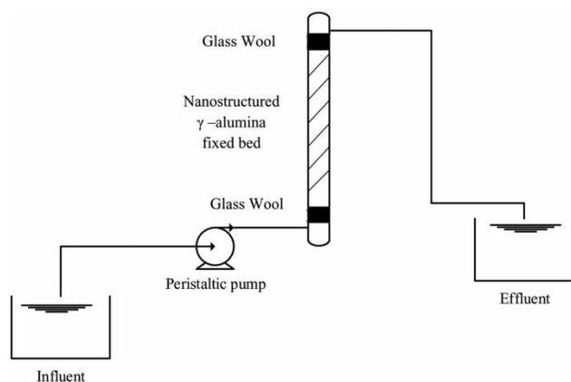
Figure 1 | Schematic diagram of the experimental column.
