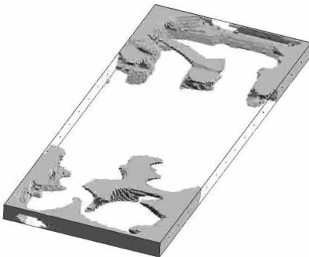
Figure 7 | Simulation of a pool tank showing areas of the pool with >70% original water after 6 hours.
