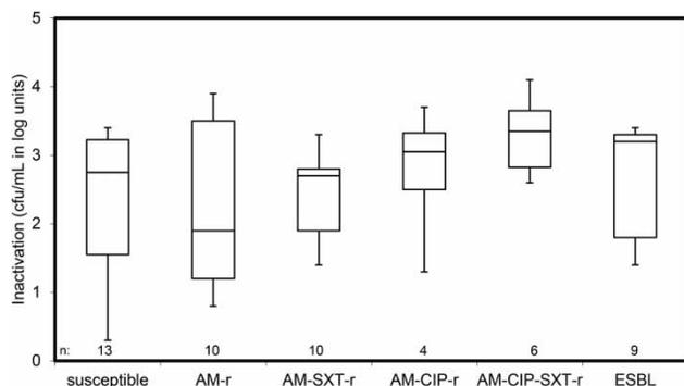
**Figure 2** | Inactivation of 13 antibiotic susceptible and 39 antibiotic resistant *E. coli* strains that were isolated from sewage and river water samples after inactivation by 4 mg/L ozone for 5 minutes. Number of tested isolates, n; resistant strains against ampicillin (AM-r), cotrimoxazol (SXT-r), ciprofloxacin (CIP-r) and extended-spectrum- $\beta$ -lactamase producers (ESBL).
