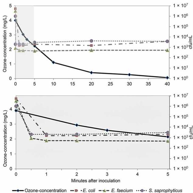
**Figure 1** | Decrease of the ozone concentration and of colony forming units in an *E. coli*, *E. faecium* and *S. saprophyticus* culture in the presence of initially 4 mg/L ozone. Mean of four analyses of ozone and of two analyses of bacterial densities for each sample.
