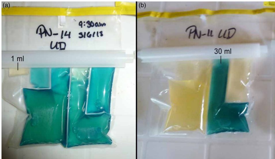
Figure 2 | Examples of positive and negative results that can be seen when running a CBT. Blue indicates the compartment is positive for E. coli and yellow indicates it is negative. Photograph (a) shows a test where all compartments except the 1 ml were positive, photograph (b) is a test where only the 30 ml compartment was positive. Please refer to the online version of this paper to see this figure in color.
