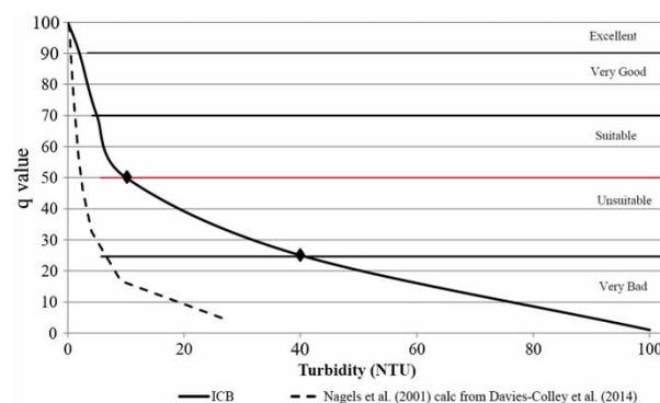
**Figure 3** | Suitability-for-use curve for turbidity (solid curve;  $q = 0.015x^2 - 2.37x + 88.6$ ). The curve is 'anchored' by two points (marked) as discussed in the text. The suitability-for-use curve proposed by Nagels *et al.* (2001) for visual clarity (transformed to turbidity) is also shown (dashed curve).
