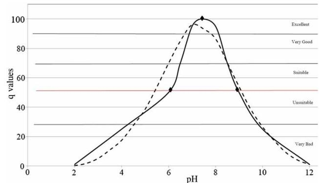
**Figure 4** | Suitability-for-use curve ( $q$ ) for pH (solid curve;  $q = -0.122x^3 - 0.747x^2 + 31.23x - 64.7$ ). The curve is 'anchored' by three points discussed in the text. The suitability-for-use curve proposed by Nagels *et al.* (2001) is also shown (dashed curve).
