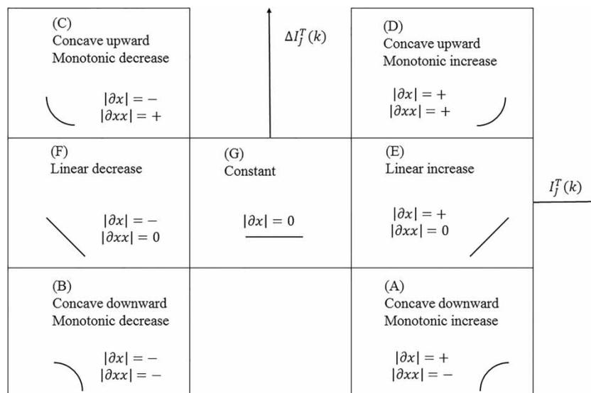
**Figure 1** | Triangular episodic representation defined by the index  $I_j^T(k)$  and the derivative  $\Delta I_j^T(k)$ : seven basic types of episodes used for interval description, each episode type is denoted by a letter from the set from A to G (redrawn from Kivikunnas 1999; Juuso 2011).
