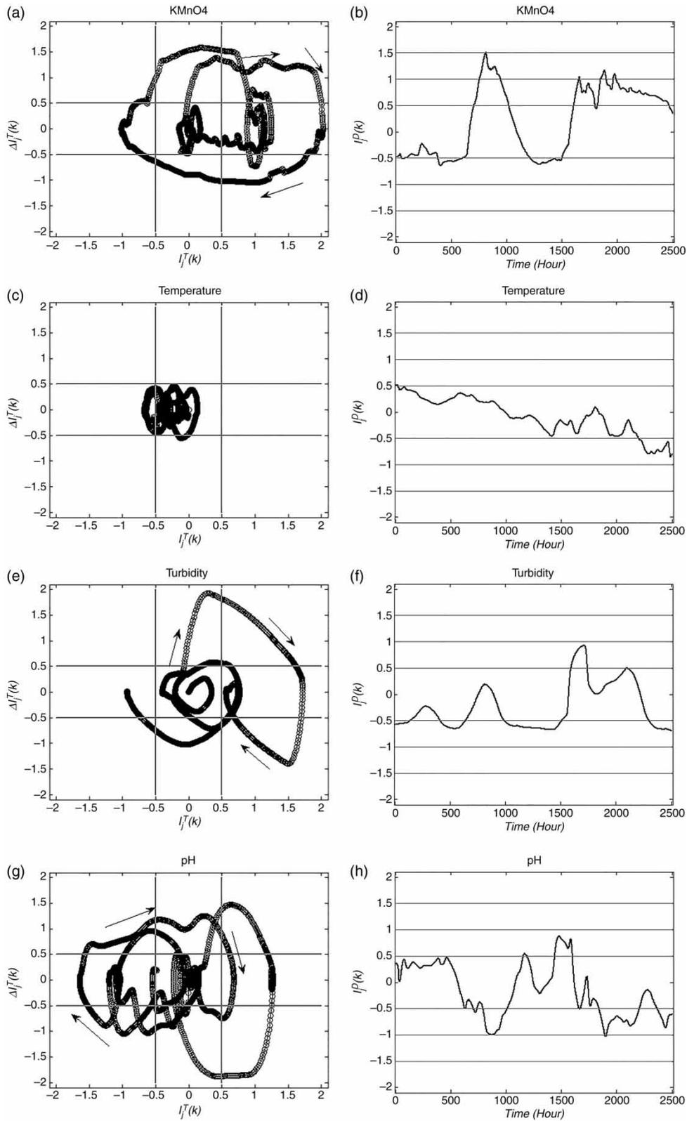
**Figure 6** | Trend episodes (left) and deviation indices (right) for operating conditions of water treatment: KMnO<sub>4</sub> level, the temperature, turbidity and pH of raw water.
