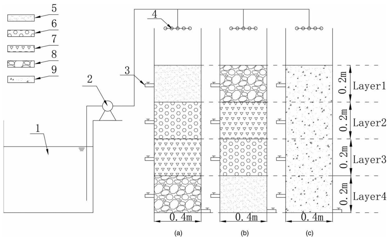
**Figure 1** | Schematic description of eco-soil reactor with different media filling schemes. (a) I-filling; (b) D-filling; (c) B-filling. 1, tank; 2, peristaltic pump; 3, sample connection; 4, water distributor; 5, grit; 6, zeolite; 7, limestone; 8, gravel; 9, blend.
