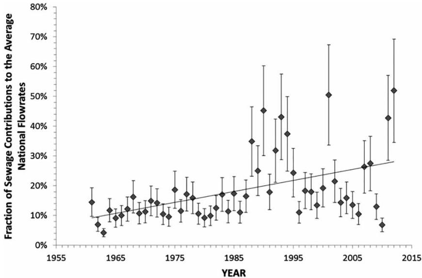
**Figure 4** | Estimated fraction of sewage contribution to the average national flow rates in the Republic of Macedonia during the period 1961–2012. Error bars represent sewage discharges rates of 150 and 300 L/capita/day used as low- and high-end values.
