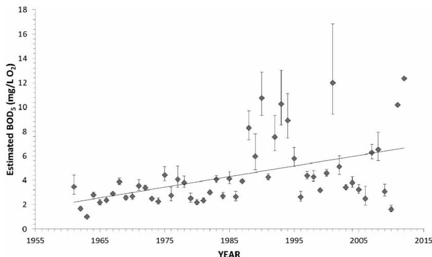
**Figure 6** | Modeled BOD estimates as an indicator of the surface water quality impairment resulting from direct sewage discharge into Macedonian rivers. The error bars represent one standard deviation boundaries.
