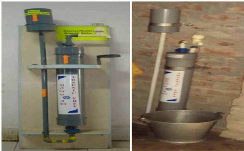
**Figure 3** | Wall mounted household ATUs, devised by Council of Scientific & Industrial Research, Central Salt & Marine Chemical Research laboratory were provided in Sangrampur, Merudandi and Basirhat areas in West Bengal State during 2009. *Source:* P. S. Anand (2013). Approaches to arsenic removal from drinking water sources and learning from field experiences. Workshop on Arsenic Removal Technologies, organized by Ministry of Environment & Forest, Government of India, Kolkata.
