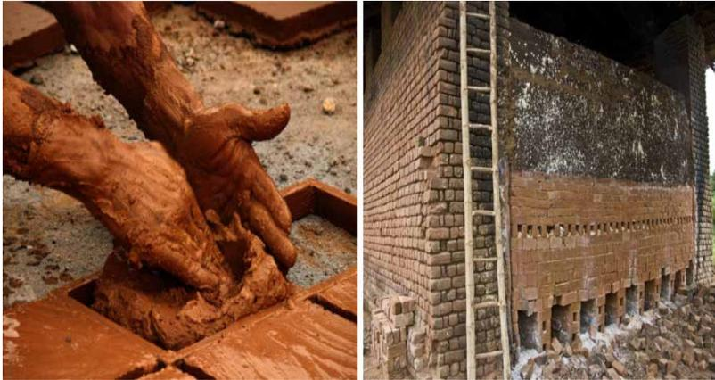
**Figure 5** | Towards safe disposal of arsenic containing sludge: use of arsenic containing sludge in making bricks. *Source:* Presentation in Workshop on Arsenic Removal Technologies. Organized by MoEF, Government of India, Kolkata (2013).
