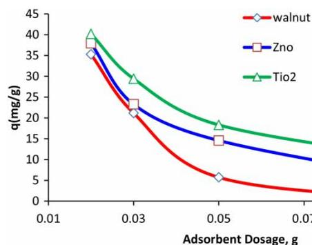
**Figure 8** | Effect of adsorbent dose on the adsorption capacity of the three adsorbents (Walnut shell adsorbent at concentration of 30 mg/L of humic acid and contact time 10 min, walnut shell modified with TiO<sub>2</sub> at concentration of 30 mg/L of humic acid and contact time 30 min, and walnut shell modified with ZnO at concentration of 10 mg/L of humic acid and contact time 10 min).
