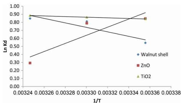
**Figure 9** | Effect of temperature on adsorption of humic acid by walnut shell, walnut shell modified with TiO<sub>2</sub>, and walnut shell modified with ZnO.
