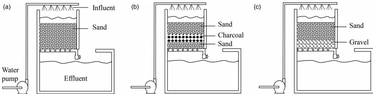
**Figure 3** | Cross-sectional graphs of household sand filters used in Ha Nam, North Vietnam. Schemas for three kinds of sand filters composed of sand (a), sand and charcoal (b), and sand and gravel (c) are presented.
