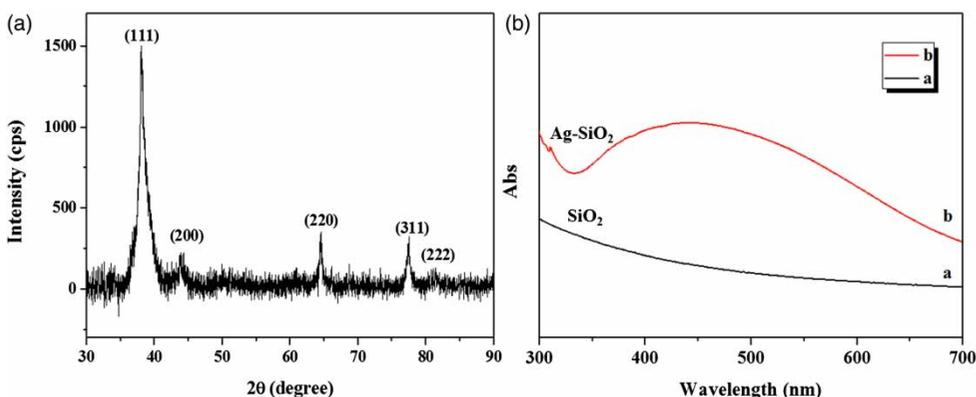
**Figure 2** | (a) XRD pattern of Ag-SiO<sub>2</sub>; (b) UV-visible absorption spectra of bare silica particles and Ag-SiO<sub>2</sub> nanohybrid.
