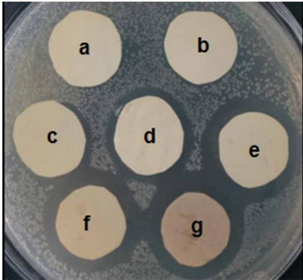
**Figure 8** | The anti-bacterial results for *E. coli* on the different membranes: (a) pure PSf membrane; (b) SiO<sub>2</sub>/PSf hybrid membrane with 0.45 wt% SiO<sub>2</sub>; Ag-SiO<sub>2</sub>/PSf hybrid with different contents of Ag-SiO<sub>2</sub>: (c) 0.15 wt%, (d) 0.3 wt%, (e) 0.45 wt%, (f) 0.6 wt%, (g) 0.75 wt%.
