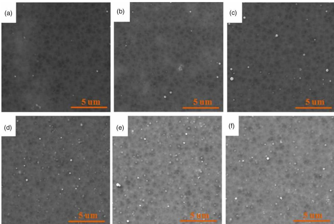
**Figure 6** | SEM images of the surfaces of Ag-SiO<sub>2</sub>/PSf hybrid membranes with different contents of Ag-SiO<sub>2</sub>: (a) 0 wt%; (b) 0.15 wt%; (c) 0.3 wt%; (d) 0.45 wt%; (e) 0.60 wt%; (f) 0.75 wt%.
