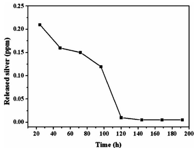
Figure 10 | The silver release measurement of Ag-SiO<sub>2</sub>/PSf hybrid membrane.
