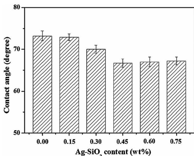
**Figure 4** | Contact angles of Ag-SiO<sub>2</sub>/PSf hybrid membranes against water as a function of Ag-SiO<sub>2</sub> content in the casting solution.
