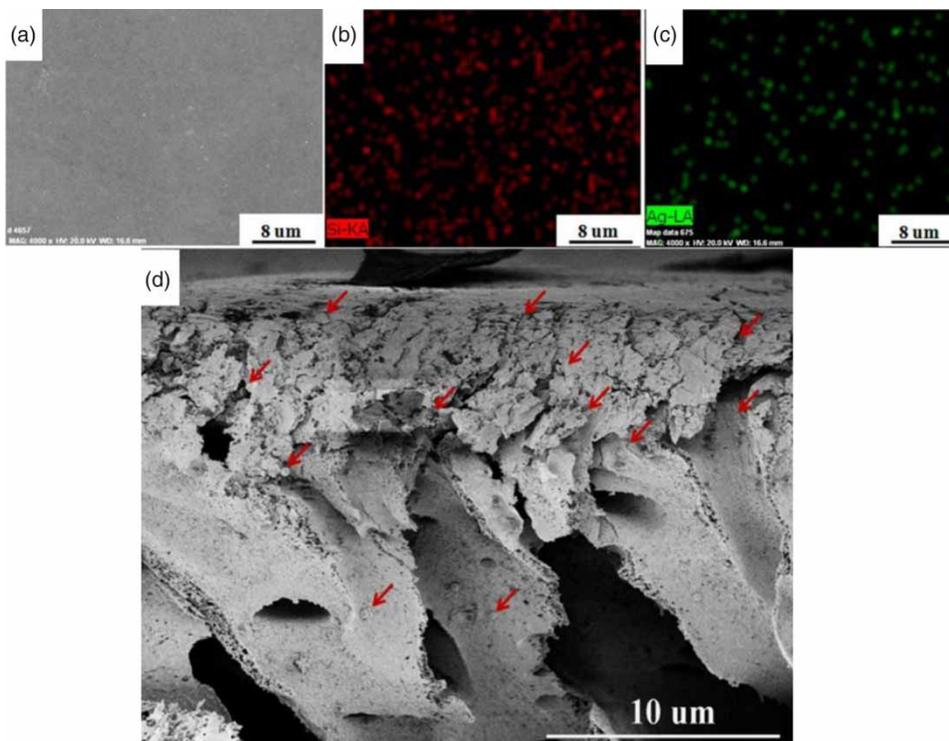
**Figure 9** | (a) SEM image of the surface of Ag-SiO<sub>2</sub>/PSf hybrid membrane with 0.45 wt% of Ag-SiO<sub>2</sub> nanohybrid; (b) Si-mapped distribution of the corresponding membrane; (c) Ag-mapped distribution of the corresponding membrane; (d) SEM image of the cross-section of the hybrid membrane.
