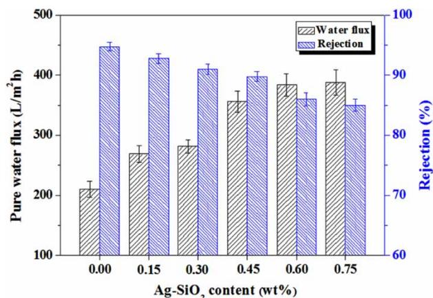
**Figure 3** | Effect of Ag-SiO<sub>2</sub> content in the casting solution on the pure water flux and rejection to egg albumin of Ag-SiO<sub>2</sub>/PSf hybrid membranes at 0.2 MPa operation pressure.
