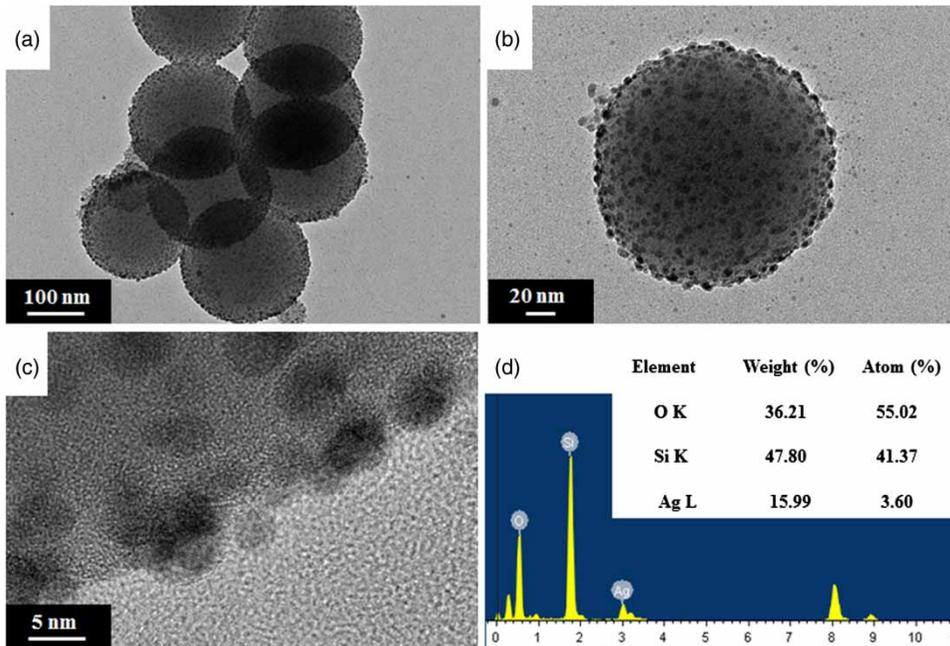
**Figure 1** | (a)–(c) TEM images of Ag-SiO<sub>2</sub> and (d) EDX spectrum of Ag-SiO<sub>2</sub>.
