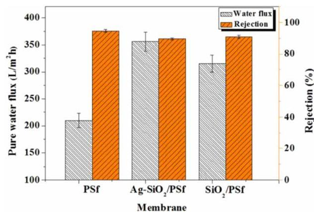
Figure 11 | Performance of membranes with different components.
