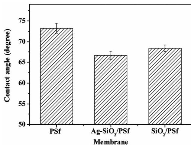
Figure 12 | Contact angles of membranes with different components.
