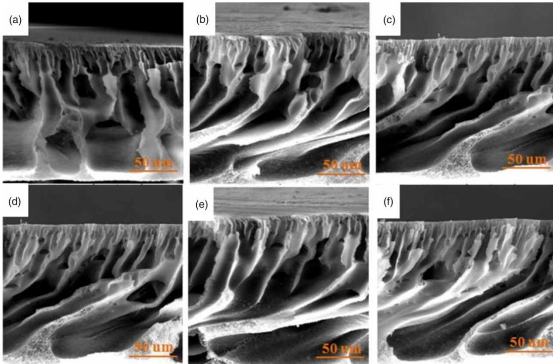
**Figure 5** | SEM images of the cross-sections of Ag-SiO<sub>2</sub>/PSf membranes with different contents of Ag-SiO<sub>2</sub>: (a) 0 wt%; (b) 0.15 wt%; (c) 0.3 wt%; (d) 0.45 wt%; (e) 0.60 wt%; (f) 0.75 wt%.
