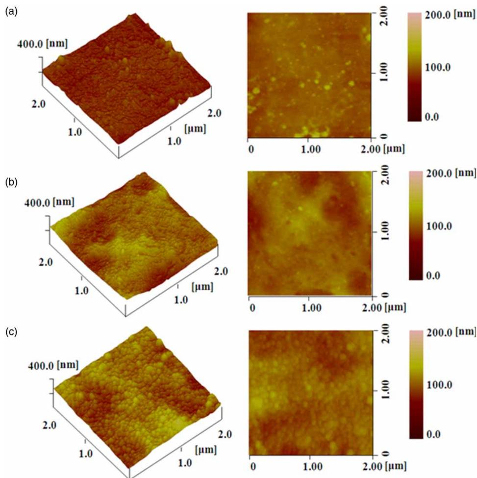
**Figure 7** | AFM images of the surfaces of the Ag-SiO<sub>2</sub>/PSf hybrid membranes with different contents of Ag-SiO<sub>2</sub>: (a) 0 wt%; (b) 0.45 wt%; (c) 0.75 wt%.
