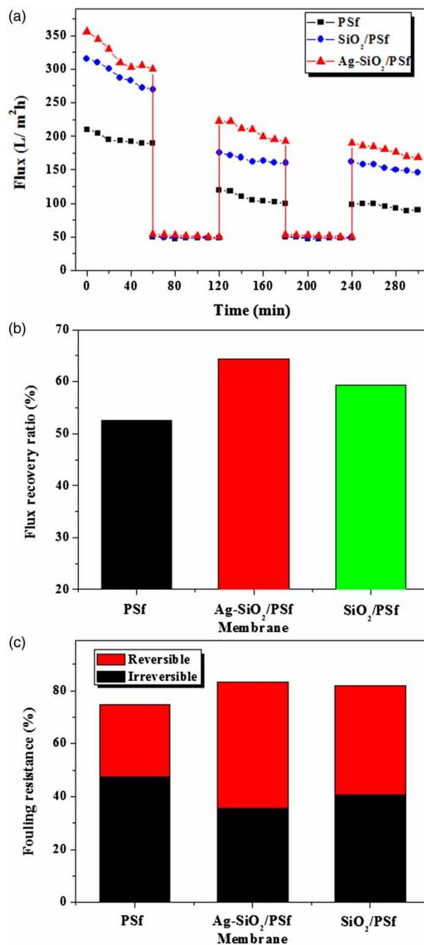
Figure 13 | (a) Time-dependent fluxes of membranes with different components during anti-fouling experiment with BSA filtration (1 mg/mL, pH = 7) at 0.2 MPa; (b) FRR of the membranes; (c) fouling resistance of the membranes.
