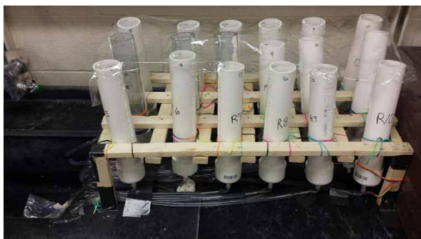
Figure 3 | Flowrate testing apparatus.
