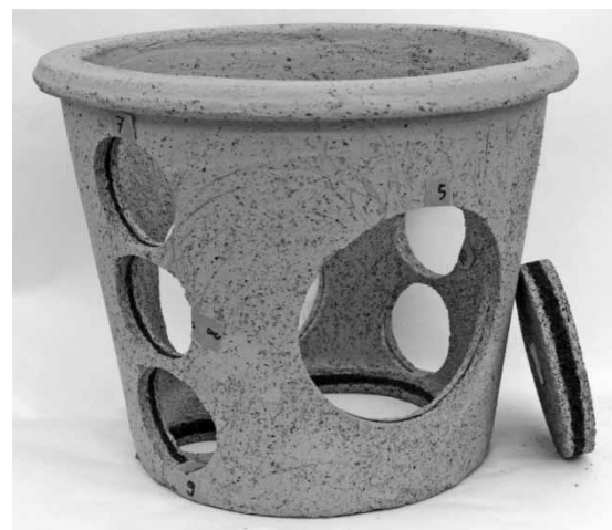
Figure 1 | Production CPF sampled to show carbon core throughout the body.
