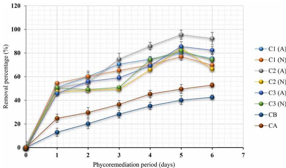
**Figure 8** | Removal of orthophosphate ( $\text{PO}_4^{3-}$ ) during the aerated (A) and non-aerated (N) phycoremediation process of public market wastewater for 6 days and with different concentrations of *Scenedesmus* sp. (C1,  $7 \log_{10} \text{ cell } 100 \text{ mL}^{-1}$ ; C2,  $8 \log_{10} \text{ cell } 100 \text{ mL}^{-1}$ ; C3  $9 \log_{10} \text{ cell } 100 \text{ mL}^{-1}$ ); control of bacteria (CB); control of algae (CA).
