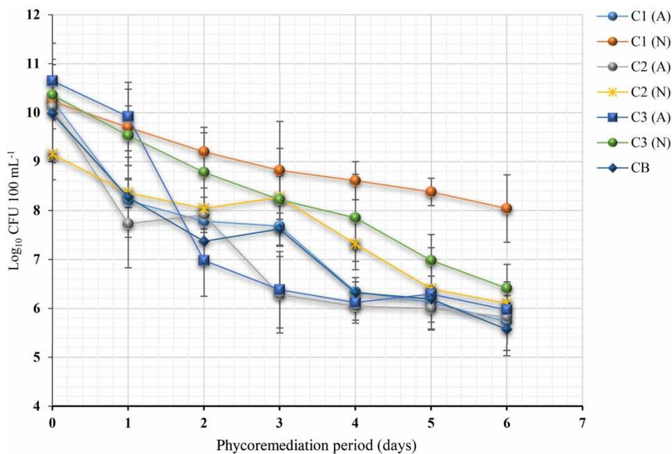
**Figure 3** | *E. faecalis* concentrations during the aerated (A) and non-aerated (N) phycoremediation process of public market wastewater for 6 days and with different concentrations of *Scenedesmus* sp. (C1,  $7 \log_{10}$  cell  $100 \text{ mL}^{-1}$ ; C2,  $8 \log_{10}$  cell  $100 \text{ mL}^{-1}$ ; C3  $9 \log_{10}$  cell  $100 \text{ mL}^{-1}$ ).
