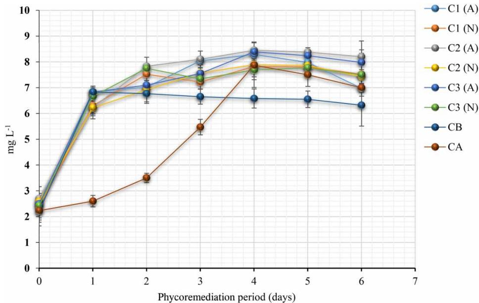
**Figure 5** | Dissolved oxygen (DO) concentrations during the aerated (A) and non-aerated (N) phycoremediation process of public market wastewater for 6 days and with different concentrations of *Scenedesmus* sp. (C1,  $7 \log_{10} \text{ cell } 100 \text{ mL}^{-1}$ ; C2,  $8 \log_{10} \text{ cell } 100 \text{ mL}^{-1}$ ; C3  $9 \log_{10} \text{ cell } 100 \text{ mL}^{-1}$ ); control of bacteria (CB); control of algae (CA).
