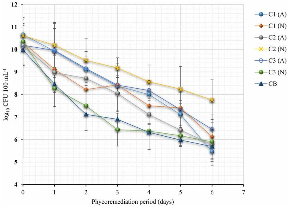
**Figure 1** | *Staphylococcus aureus* concentrations during the aerated (A) and non-aerated (N) phycoremediation process of public market wastewater for 6 days and with different concentrations of *Scenedesmus* sp. (C1, 7 log<sub>10</sub> cell 100 mL<sup>-1</sup>; C2, 8 log<sub>10</sub> cell 100 mL<sup>-1</sup>; C3 9 log<sub>10</sub> cell 100 mL<sup>-1</sup>); control (CB).
