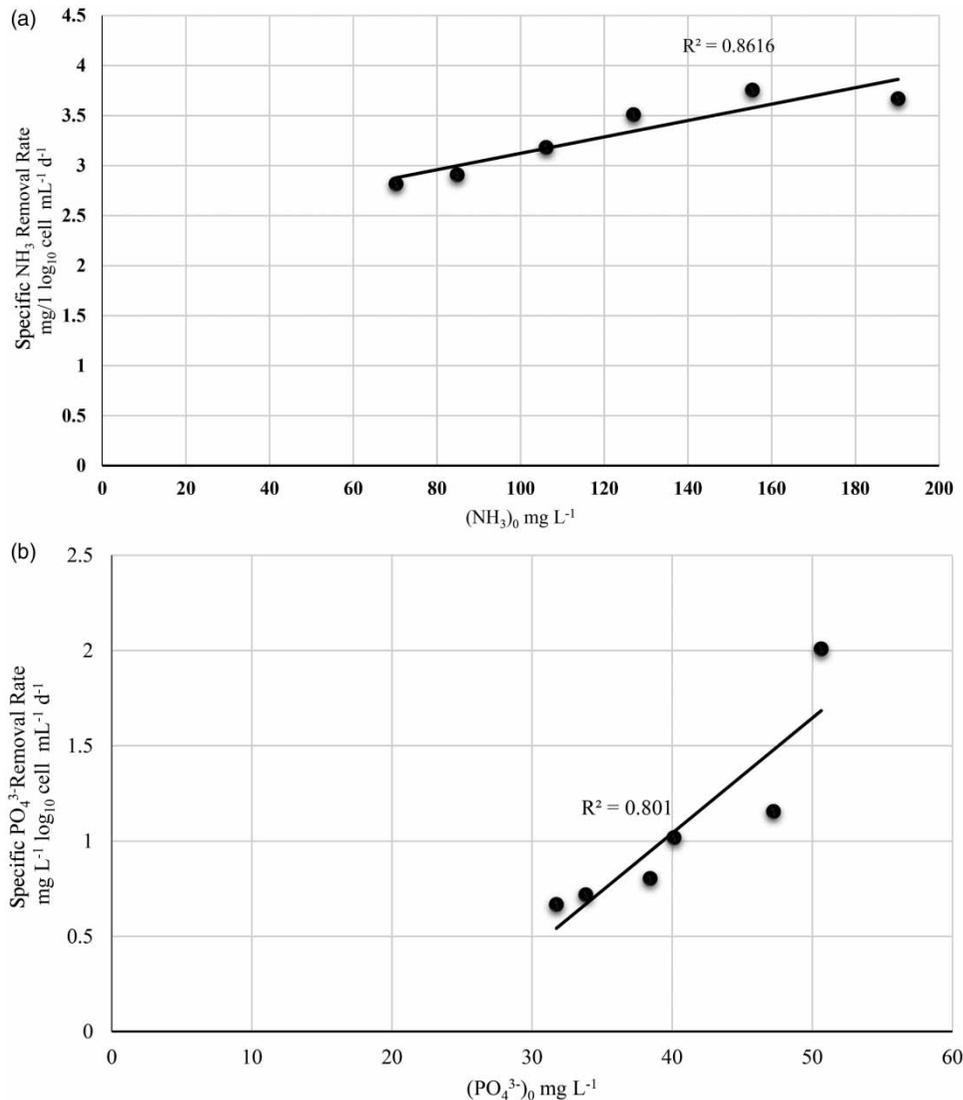
**Figure 9** | (a) Effect of initial concentration of  $\text{NH}_3$  on the specific removal by *Scenedesmus* sp. with initial concentrations of  $8 \log_{10}$  cell  $\text{mL}^{-1}$ . (b) Effect of initial concentration of  $\text{PO}_4^{3-}$  on the specific removal by *Scenedesmus* sp. with initial concentrations of  $8 \log_{10}$  cell  $\text{mL}^{-1}$ .
