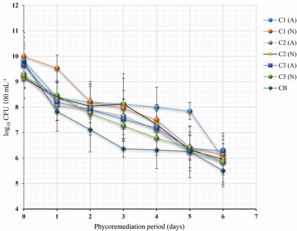
**Figure 2** | *E. coli* concentrations during the aerated (A) and non-aerated (N) phycoremediation process of public market wastewater for 6 days and with different concentrations of *Scenedesmus* sp. (C1, 7 log<sub>10</sub> cell 100 mL<sup>-1</sup>; C2, 8 log<sub>10</sub> cell 100 mL<sup>-1</sup>; C3 9 log<sub>10</sub> cell 100 mL<sup>-1</sup>); control (CB).
