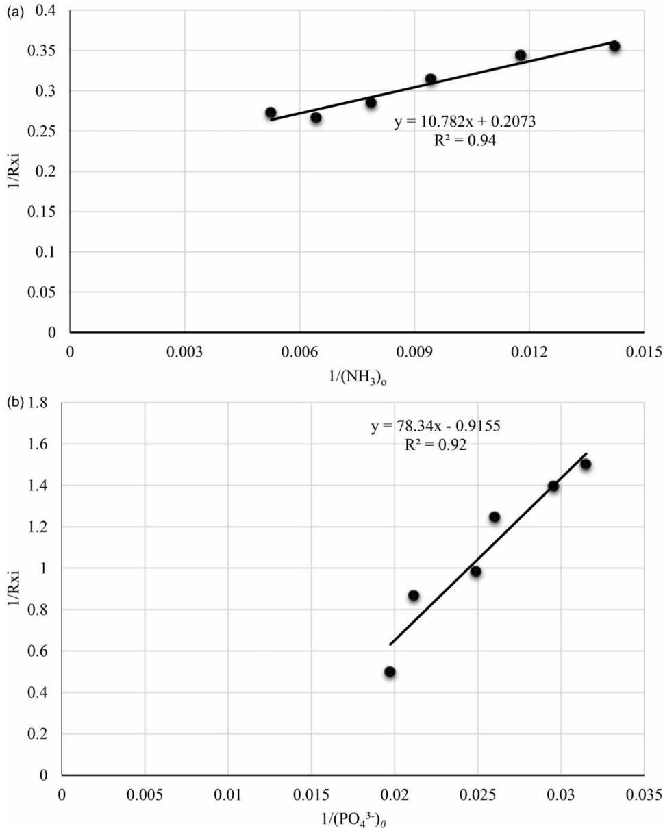
**Figure 11** | (a) Effect of  $\text{NH}_3$  concentrations on specific removal rate by *Scenedesmus* sp.  $k = 4.82$ ,  $k_m = 52$ . (b) Effect of  $\text{PO}_4^{3-}$  concentrations on specific removal rate by *Scenedesmus* sp.  $k = 1.09$ ,  $k_m = 85.56$ .
