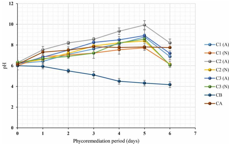
**Figure 6** | pH values during the aerated (A) and non-aerated (N) phycoremediation process of public market wastewater for 6 days and with different concentrations of *Scenedesmus* sp. (C1,  $7 \log_{10}$  cell  $100 \text{ mL}^{-1}$ ; C2,  $8 \log_{10}$  cell  $100 \text{ mL}^{-1}$ ; C3  $9 \log_{10}$  cell  $100 \text{ mL}^{-1}$ ), control of bacteria (CB); control of algae (CA).
