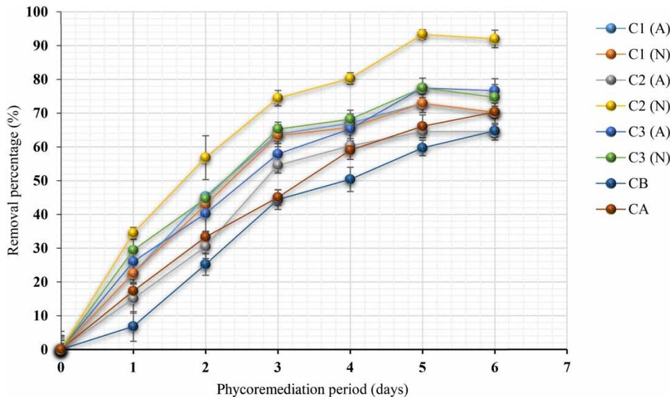
**Figure 7** | Removal of ammonium ( $\text{NH}_4^+$ ) during the aerated (A) and non-aerated (N) phycoremediation process of public market wastewater for 6 days and with different concentrations of *Scenedesmus* sp. (C1,  $7 \log_{10}$  cell  $100 \text{ mL}^{-1}$ ; C2,  $8 \log_{10}$  cell  $100 \text{ mL}^{-1}$ ; C3  $9 \log_{10}$  cell  $100 \text{ mL}^{-1}$ ); control of bacteria (CB); control of algae (CA).
