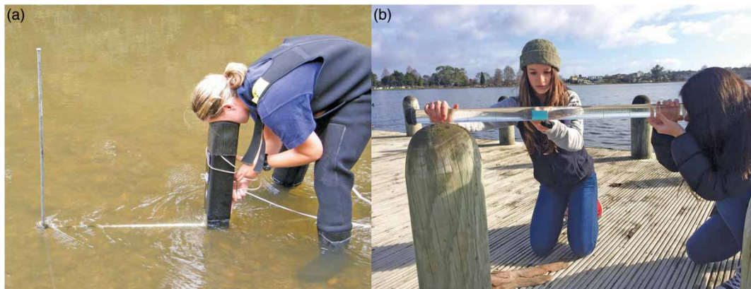
Figure 1 | Measurement of visual water clarity by the black disc method. (a) Visual clarity measurement in situ as the horizontal sighting range of a black disc. The observer is using an underwater periscope fitted with a 45° mirror to observe the horizontal extinction distance of the black target (60 mm diameter disc) fixed to a steel stake driven into the streambed. (b) The SHMAK clarity tube for water of relatively low clarity. The black target (20 mm diameter disc) is mounted on an aquarium magnet that is being moved to the extinction distance by the observer's assistant. (Photo credits: (a) Graham Timpany, NIWA; (b) Rebecca Stott, NIWA.) Please refer to the online version of this paper to see this figure in colour: http://dx.doi.org/10.2166/wh.2018.214 .
