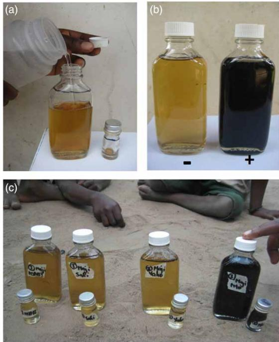
**Figure 1** | H<sub>2</sub>S water quality testing: (a) water sample being added to 100 mL and 5 mL bottles containing H<sub>2</sub>S media; (b) after 24 h at ambient temperatures (22–30 °C) positive samples turned black (bottle on the right) while negative samples had no colour change and remained straw coloured (bottle on the left); (c) H<sub>2</sub>S demonstration in the field with a community member correctly identifying the positive sample (far right).
