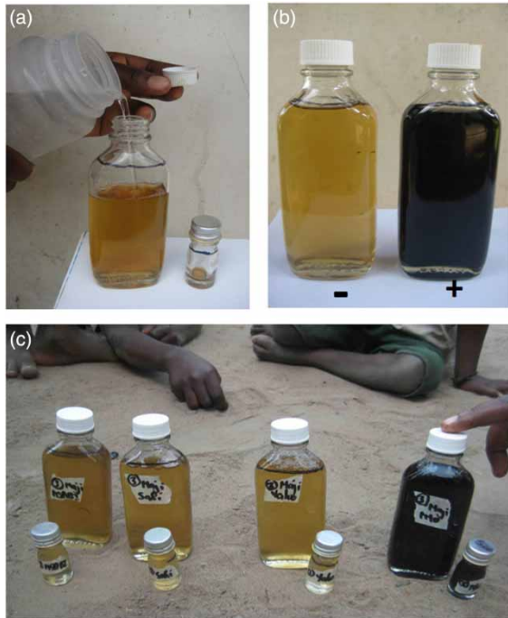
Figure 1 | H 2 S water quality testing: (a) water sample being added to 100 mL and 5 mL bottles containing H 2 S media; (b) after 24 h at ambient temperatures (22–30 °C) positive samples turned black (bottle on the right) while negative samples had no colour change and remained straw coloured (bottle on the left); (c) H 2 S demonstration in the field with a community member correctly identifying the positive sample (far right).
