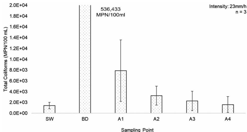
**Figure 7** | Total coliforms for the water used in the experiment (SW), the water collected before diversion (BD), and for water collected after diverting the 1st (A1), 2nd (A2), 3rd (A3), and 4th (A4) millimeters of rainwater (precipitation intensity of 23 mm/h). The error bars represent the standard deviation.
