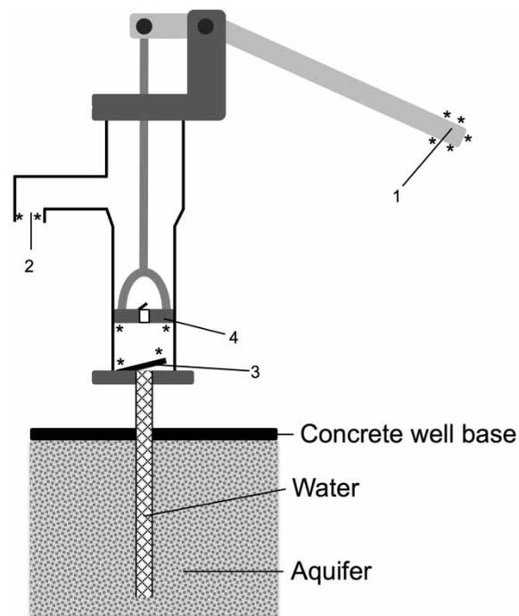
**Figure 1** | Schematic of typical suction mode hand pump. Sampling positions of well-heads. Handle: 1; spout: 2; seal: 3; piston: 4. The handle, spout and bottom of the piston are all made from metal while the seal is made from plastic. The piston assembly comprises a rubber plug, which seals the pump barrel, and a metal base. \*Indicates positions that were swabbed.
