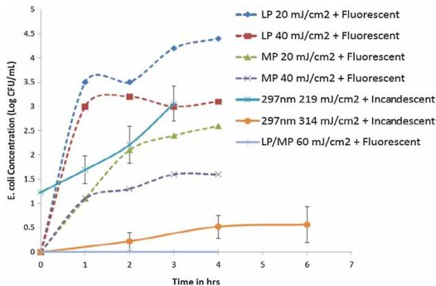
**Figure 8** | *E. coli* ATCC 15597 photorepair compared with repair caused by LP and MP lamps (LP and MP data were extracted from Quek & Hu (2008a)). Note: Error bars show standard deviation around the mean.
