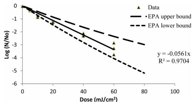
**Figure 3** | Dose-response behavior for coliphage MS2 at 254 nm. Upper and lower bounds for UV<sub>254</sub> dose-response behavior of MS2, as defined by USEPA (2006) are included for reference.
