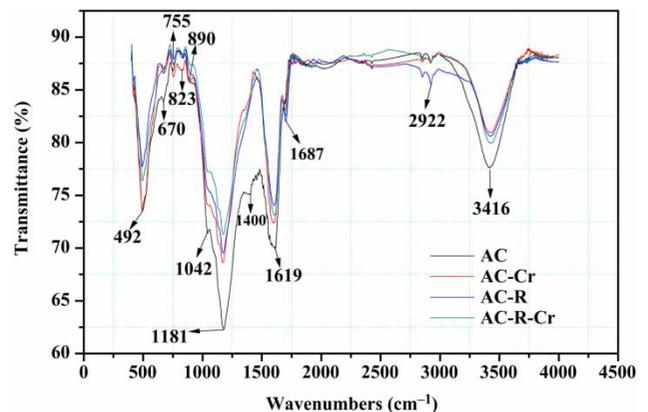
**Figure 7** | FTIR spectra of AC, AC-Cr, AC-R and AC-R-Cr.
