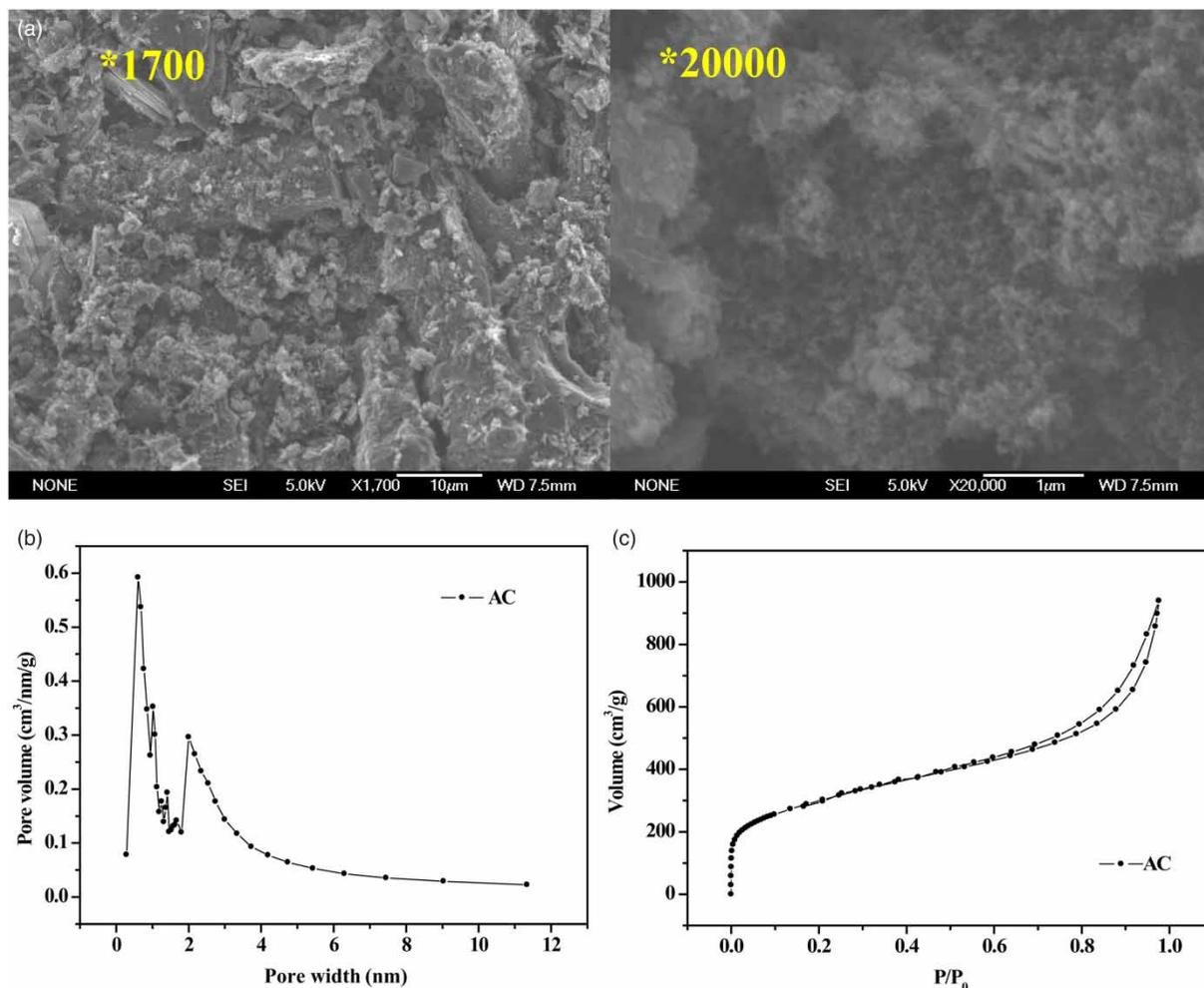
**Figure 2** | (a) SEM images, (b) pore size distribution and (c) N<sub>2</sub> adsorption/desorption isotherm of AC.
