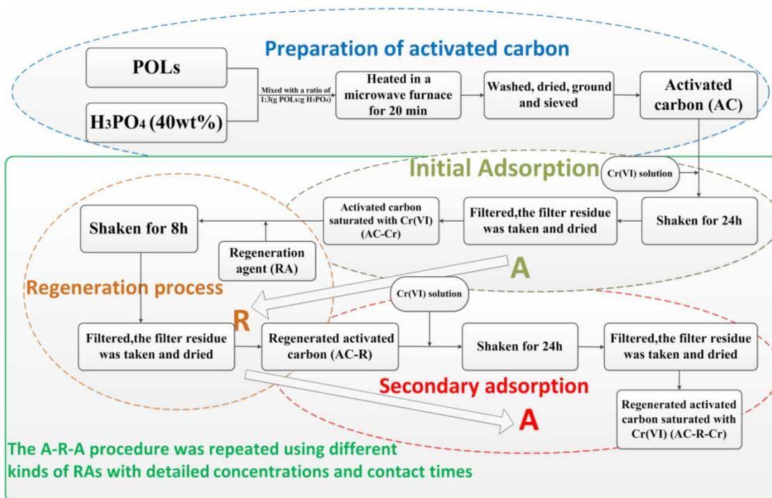
Figure 1 | The flow charts of the experimental procedure in this study.
