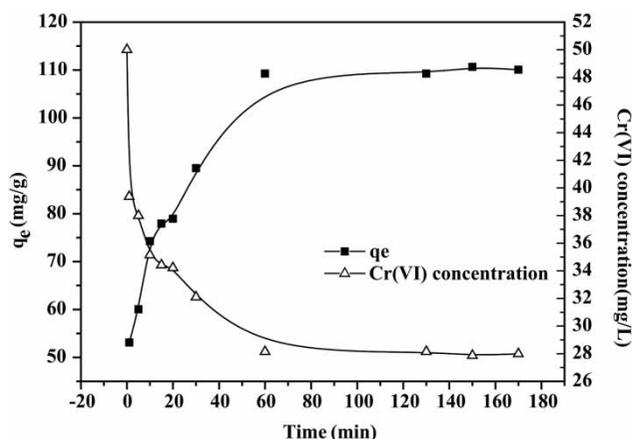
**Figure 4** | Effect of contact time on Cr(VI) adsorption (initial Cr(VI) concentration: 50 mg/L, AC dosage: 1.0 g/L, initial pH: 2.5, temperature: 25 °C).
