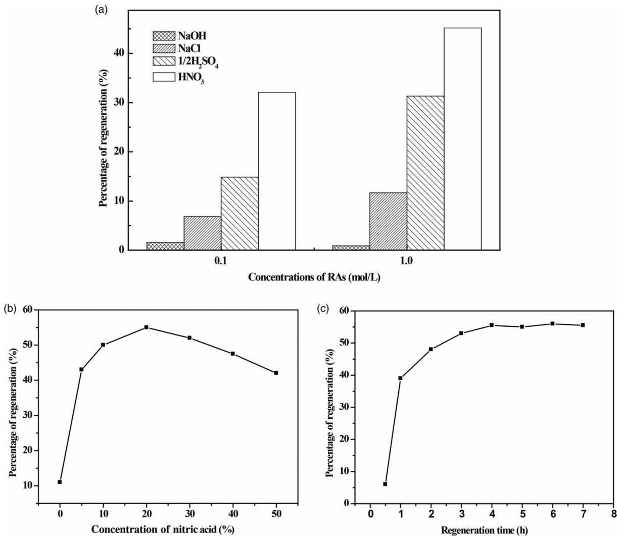
**Figure 6** | (a) Regeneration performances of HNO<sub>3</sub>, 1/2H<sub>2</sub>SO<sub>4</sub>, NaOH and NaCl after one regeneration cycle, (b) influence of concentration of HNO<sub>3</sub> on the percentage of regeneration with five regeneration cycles and (c) influence of regeneration time on the percentage of regeneration after one regeneration cycle.
