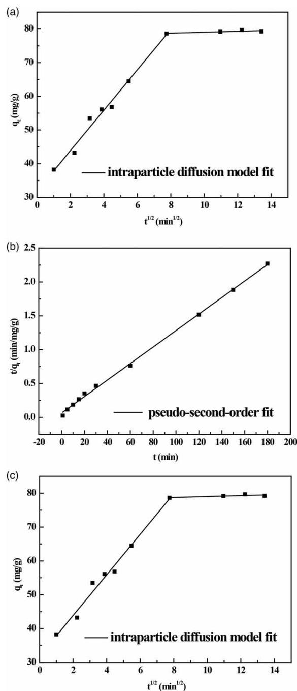
**Figure 5** | The curves of (a) pseudo-first order model, (b) pseudo-second order model and (c) intraparticle diffusion model for the removal of Cr(VI) by AC.
