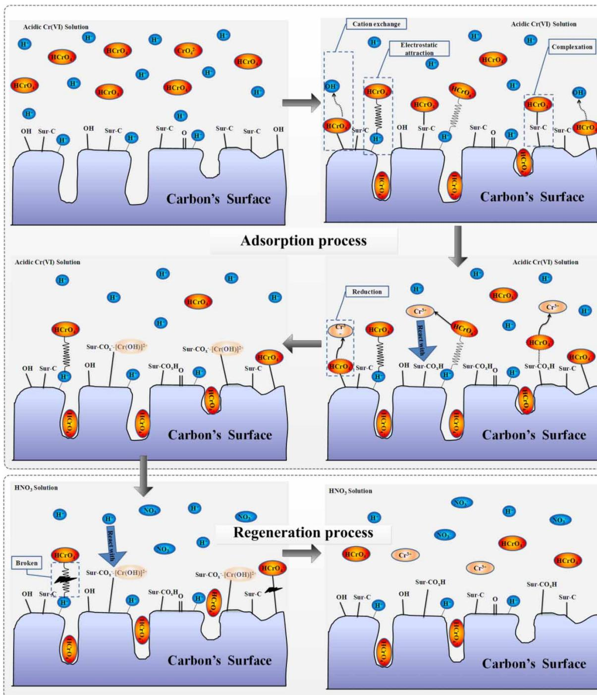
**Figure 8** | Graphical representation of the adsorption and regeneration mechanism.
