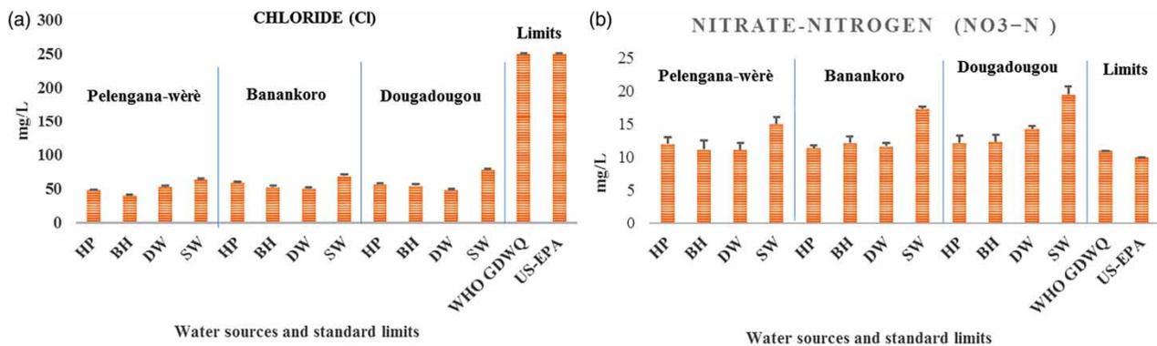
**Figure 2** | Variation of (a) Cl and (b) NO<sub>3</sub>-N in drinking water samples compared to standards.
