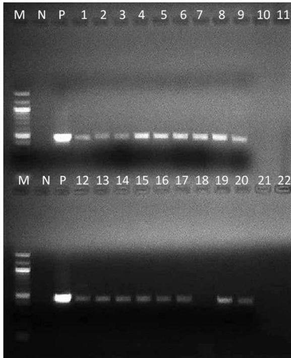
Figure 5 | The agarose gel electrophoresis of the (SSU) rDNA gene amplified by the PCR from water samples collected from Samsun province. M: 100 bp ladder, N: distilled water (negative), P: Acanthamoeba castellanii (ATCC30010), 1–22: water samples collected from the investigated areas.
