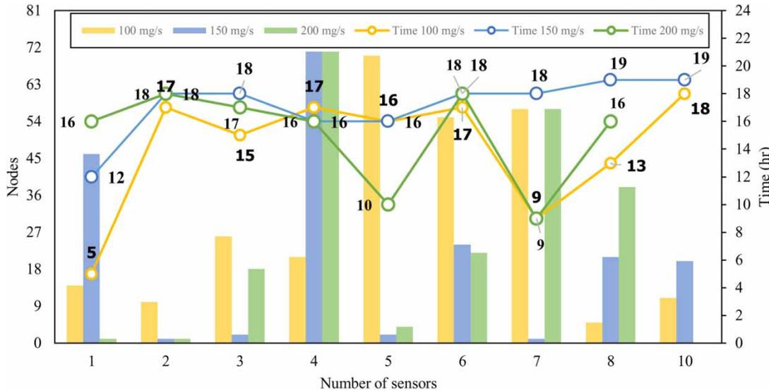
Figure 7 | The most critical time and place of injection corresponding to the number of sensors (scenarios 1–3).
