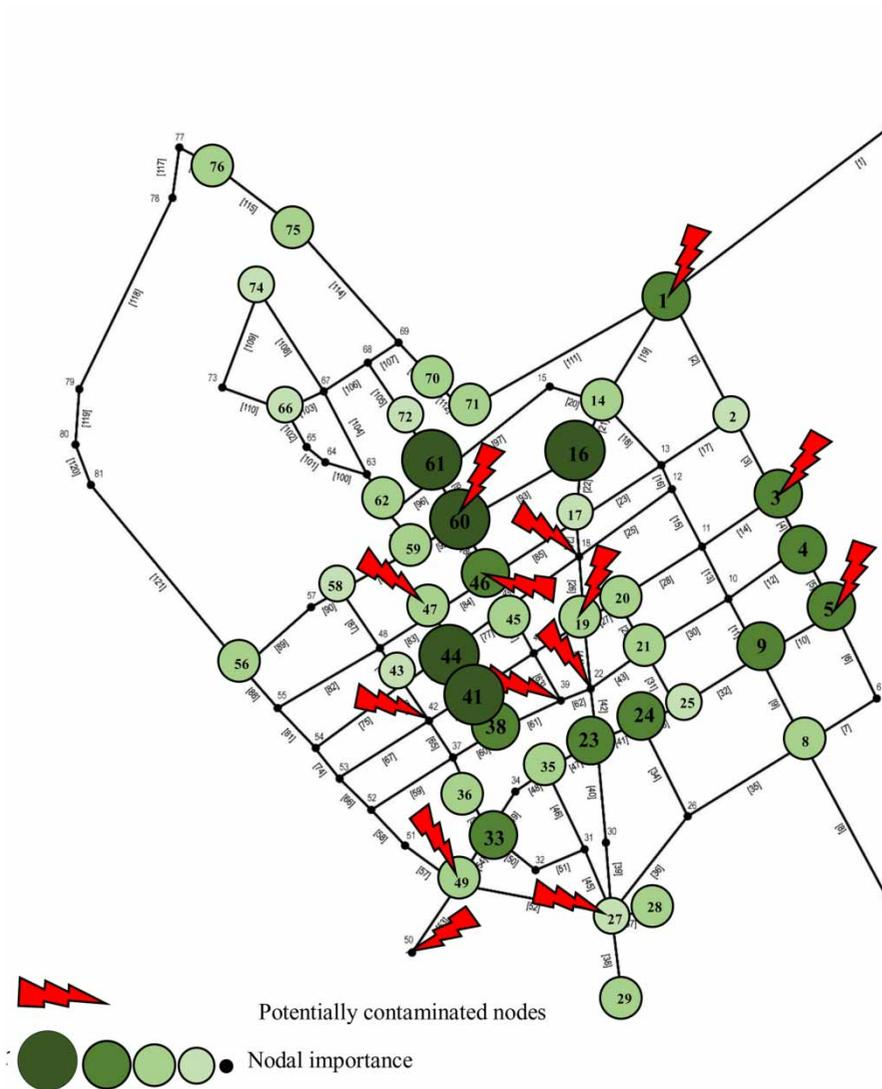
**Figure 1** | Potential locations of contamination injection.
