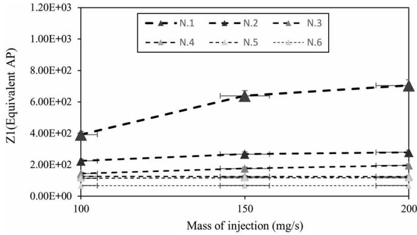
Figure 9 | Damage changes with increasing arsenic mass with number of sensors 1–6 (scenarios 4–6).
