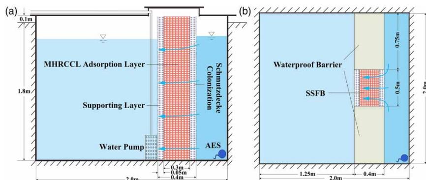
**Figure 3** | Structural schematic diagram for the M-SSF system: (a) the profile schematic diagram of the M-SSF system and (b) the plane schematic diagram of the M-SSF system.
