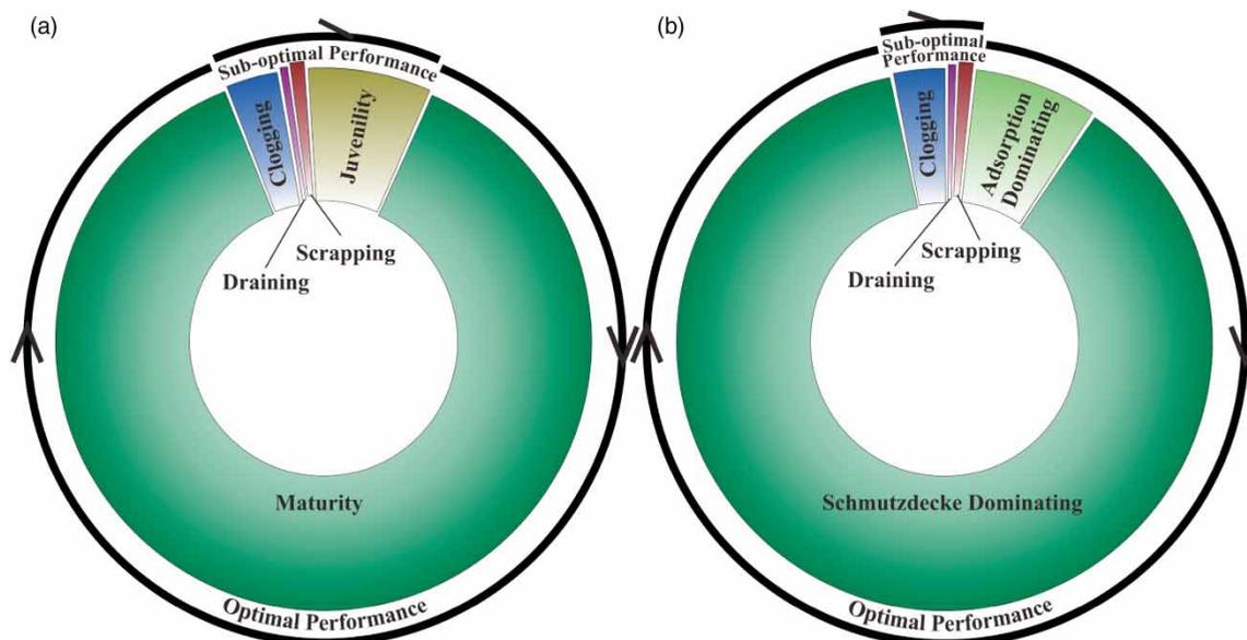
**Figure 4** | Comparison between a conventional SSF and the M-SSF system: (a) the operational period of the conventional SSF and the performance of each stage and (b) the operational period of M-SSF and the performance of each stage.
