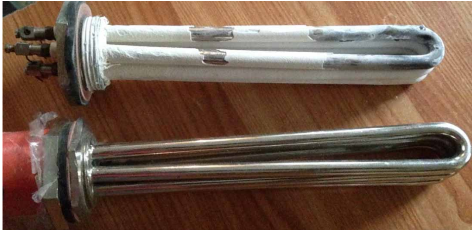
Figure 1 | An autoclave water-heating coil covered with a layer of deposits (most likely to be \text{CaCO}_3 from hard water) and a newly purchased heating coil (picture taken in one of the hospitals included in this study).
