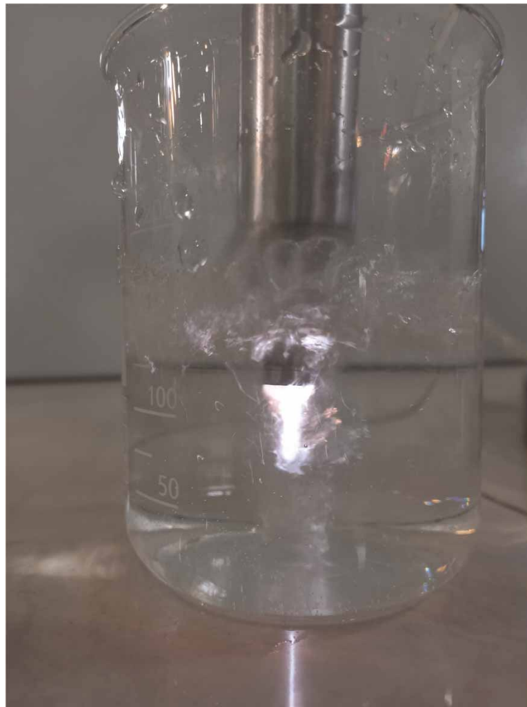
Figure 2 | Treatment of contaminated water by Argon plasma jet.
