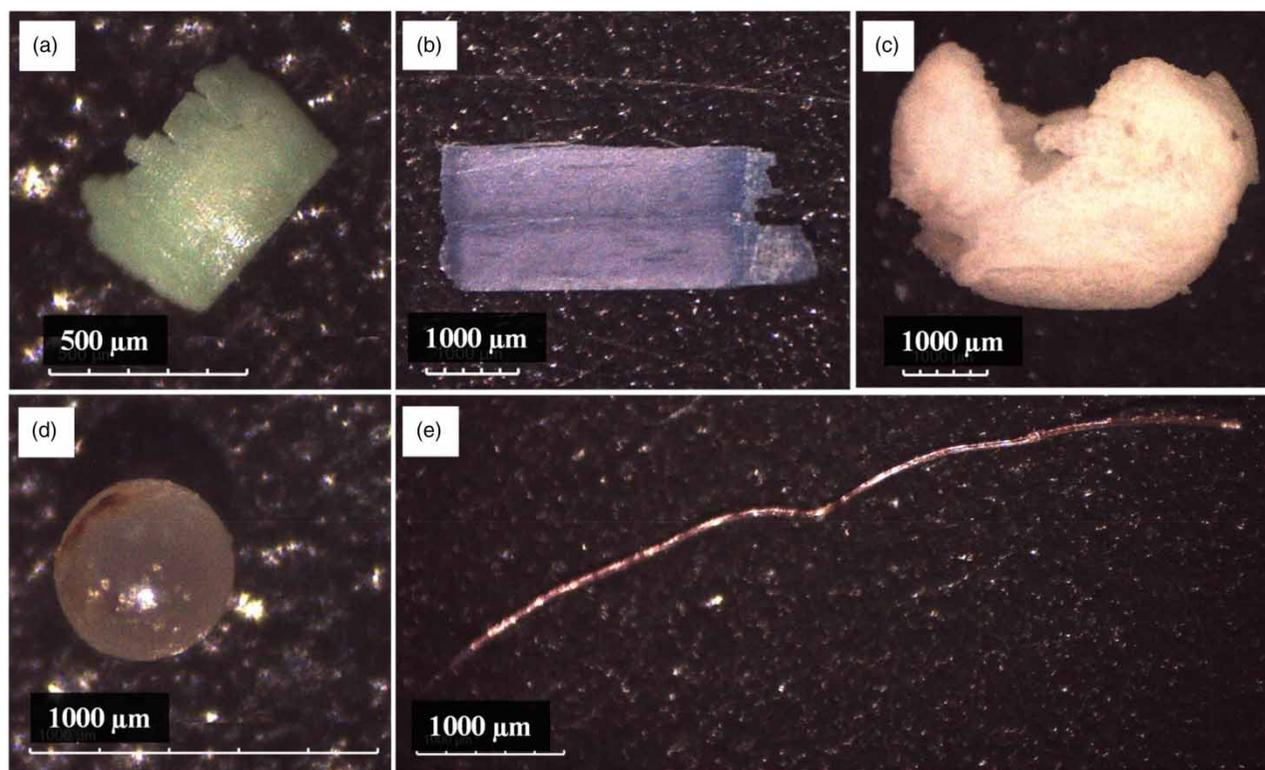
**Figure 3** | Examples of MPs in different shapes: (a) fragment; (b) sheet and film; (c) foam; (d) bead; and (e) fiber.
