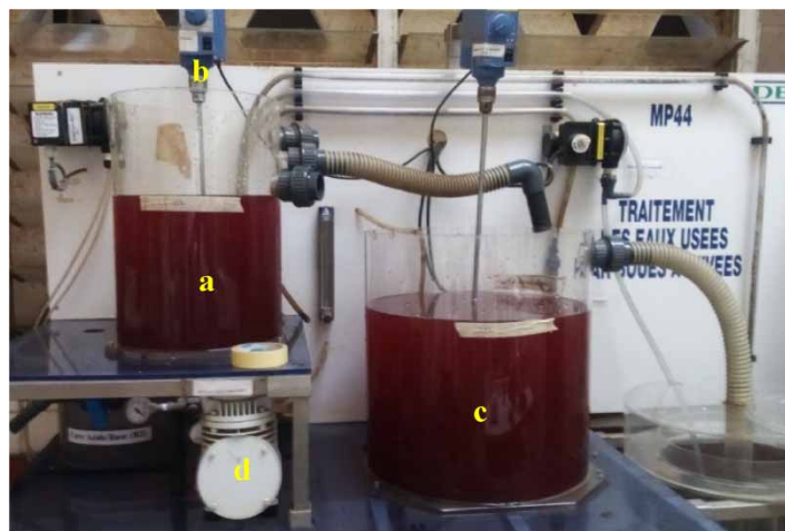
Figure 1 | Experimental design of the biological treatment process used. (a) Reactor without oxygen supply; (b) stirring blade; (c) oxygen-fed reactor; and (d) air pump.
