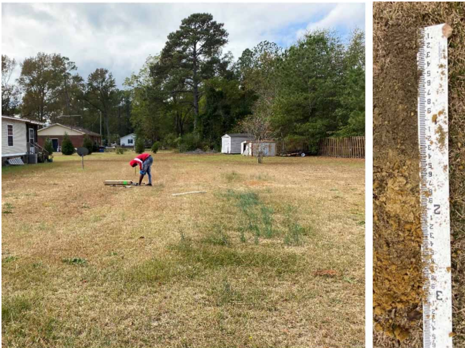
Figure 3 | Septic drainfield trenches were located using a tile-probe (left image) and soil borings near the system were laid onto the ground and characterized (right image).
