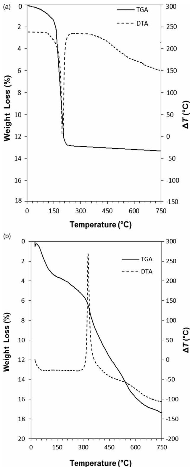
Figure 4 | TGA/DTA curves of (a) SBA-15 and (b) NH<sub>2</sub>-SBA-15.
