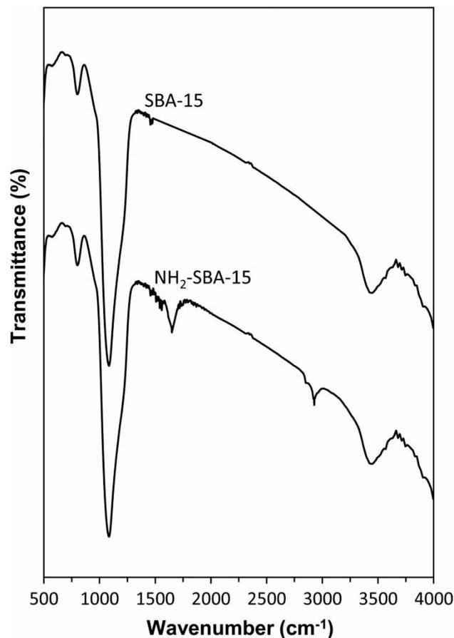
Figure 3 | FTIR spectra of SBA-15 and NH<sub>2</sub>-SBA-15.
