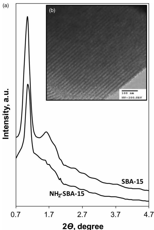
Figure 1 | (a) XRD patterns of SBA-15 and NH<sub>2</sub>-SBA-15 and (b) TEM image of SBA-15.
