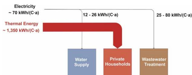
**Figure 4** | Specific energy consumption per capita (C) and year (a) in the area of urban water management, using the example of Germany; drinking water from groundwater/surface water, wastewater treatment via activated sludge process; specific water consumption approximately 120 L/(C-d) (Meda *et al.* 2012b).
