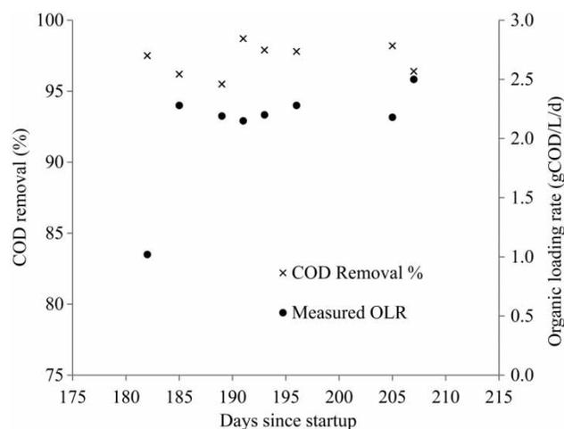
Figure 7 | COD removal during continuous operation period.
