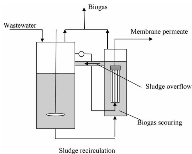
Figure 2 | Schematic of the AnMBR system.
