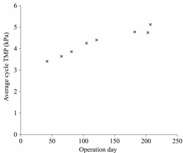
**Figure 10** | Average cycle TMP change with time
