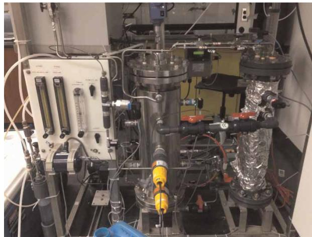
Figure 1 | AnMBR system showing digester (centre) and membrane tank (right).
