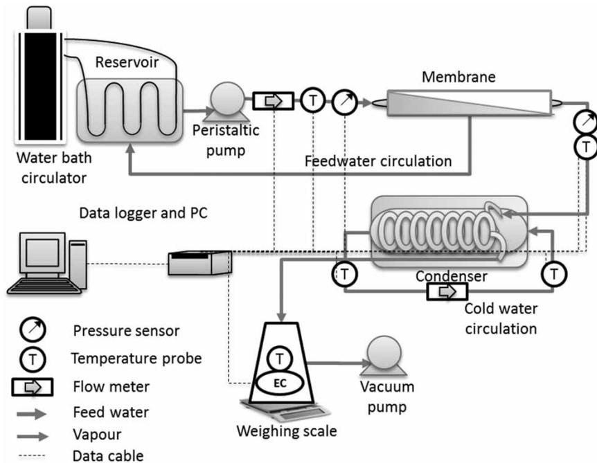
Figure 2 | VMD experimental set-up.
