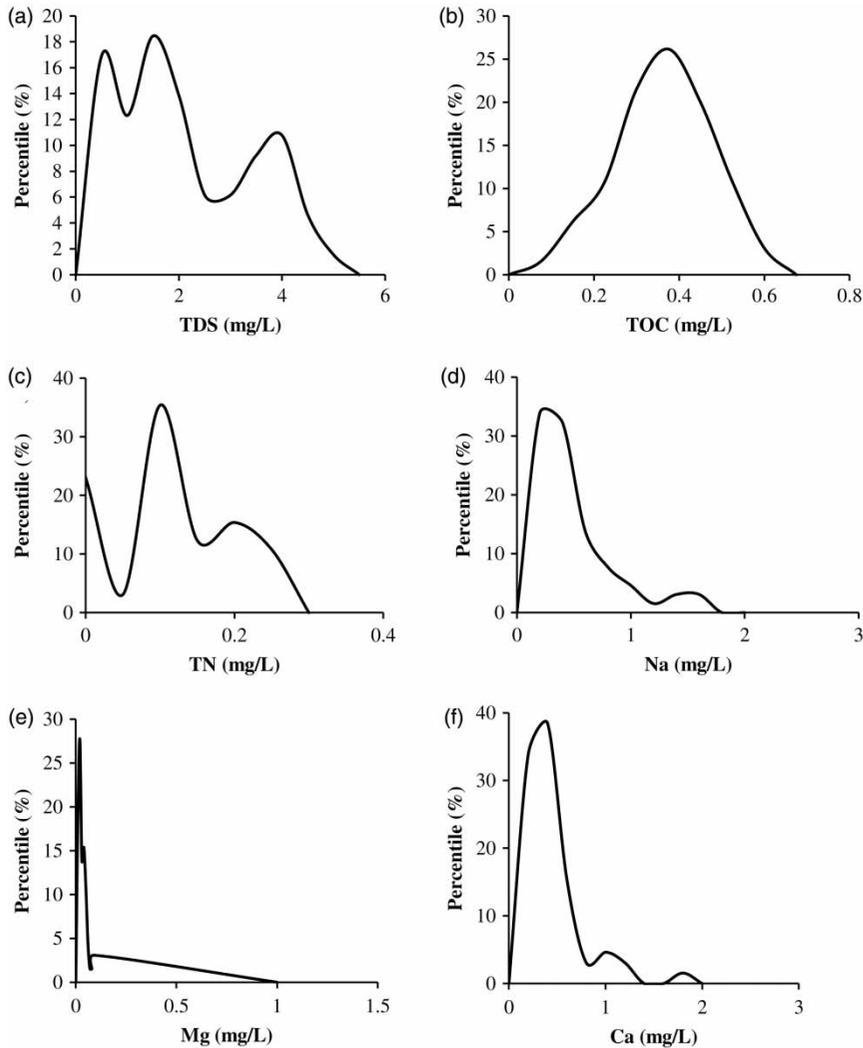
**Figure 6** | Distribution of (a) TDS, (b) TOC, (c) TN, (d) Na, (e) Mg, and (f) Ca concentration of the permeate water from VMD.
