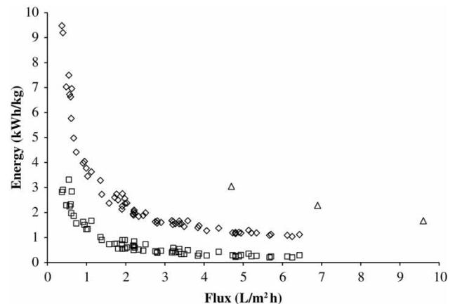
**Figure 5** | Specific energy consumption of the VMD process versus permeate flux rate. (◇) Including heat; (□) excluding heat; (Δ) Safavi & Mohammadi (2009) data.
