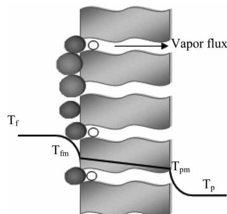
Figure 1 | Mass transfer and heat transfer through the membrane in VMD.
