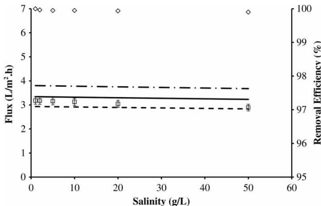
**Figure 4** | Effects of feed-water salinity on flux: (◇) modeled flux (Equation (13)); (—) modeled flux (Equation (14)); (—•—) modeled flux (Equation (15)); (□) experimental flux; (◇) removal efficiency. Temperature = 65 °C; vacuum pressure = 15 kPa; flow rate = 1 L/min.
