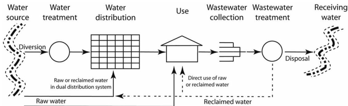
Figure 1 | Schematic of a dual water system.
