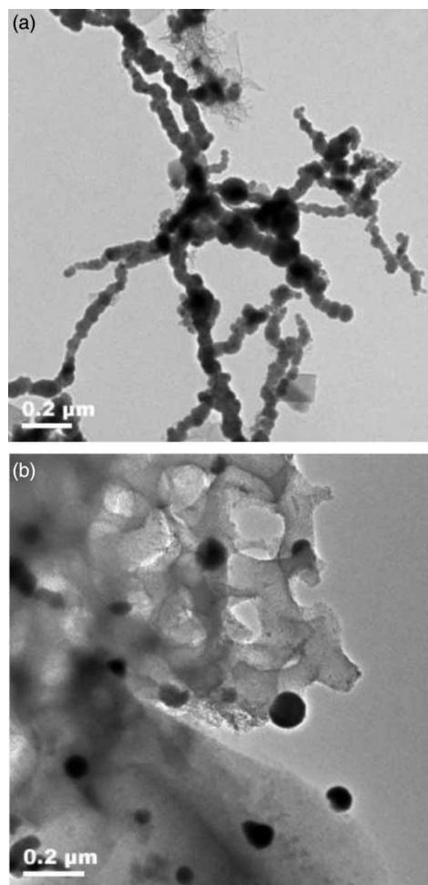
**Figure 2** | TEM images of laboratory synthesized (a) NZVI and (b) M-NZVI. The M-NZVI particles have a (MCM-41): $\text{Fe}^0$  mass ratio of 4:1.
