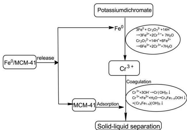
**Figure 7** | Proposed mechanism for the reduction of Cr(VI) using M-NZVI.
