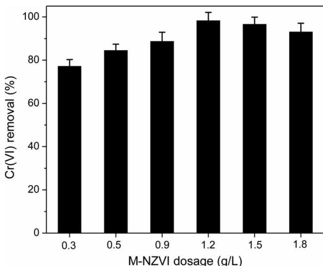
**Figure 5** | Effect of M-NZVI dosage on Cr(VI) removal by M-NZVI. The M-NZVI particles have a (MCM-41):Fe<sup>0</sup> mass ratio of 4:1. [Cr(VI)]<sub>0</sub> = 100 mg/L, reaction time = 60 min, and [pH]<sub>0</sub> = 6.0.
