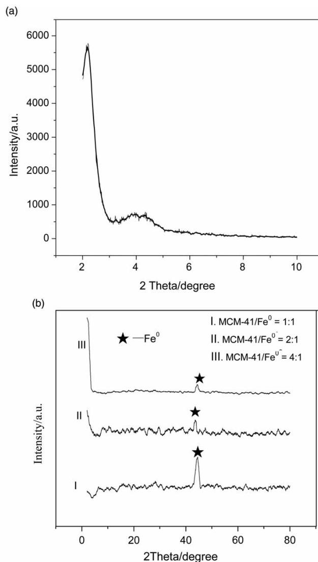
Figure 1 | XRD patterns of (a) laboratory synthesized MCM-41 and (b) M-NZVI samples.
