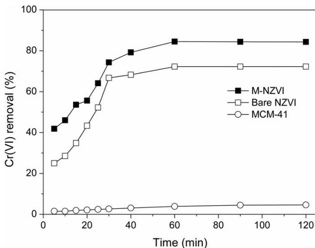
**Figure 3** | Effect of reaction time on Cr(VI) removal by MCM-41, bare NZVI, and M-NZVI. The M-NZVI particles have a (MCM-41):Fe<sup>0</sup> mass ratio of 4:1. [Cr(VI)]<sub>0</sub> = 100 mg/L, [M-NZVI]<sub>0</sub> = 0.5 g/L, [MCM-41]<sub>0</sub> = 0.4 g/L, [NZVI]<sub>0</sub> = 0.1 g/L, and [pH]<sub>0</sub> = 6.0.
