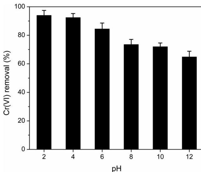
**Figure 4** | Effect of initial solution pH on Cr(VI) removal by M-NZVI. The M-NZVI particles have a (MCM-41):Fe<sup>0</sup> mass ratio of 4:1. [Cr(VI)]<sub>0</sub> = 100 mg/L, [M-NZVI]<sub>0</sub> = 0.5 g/L, and reaction time = 60 min.
