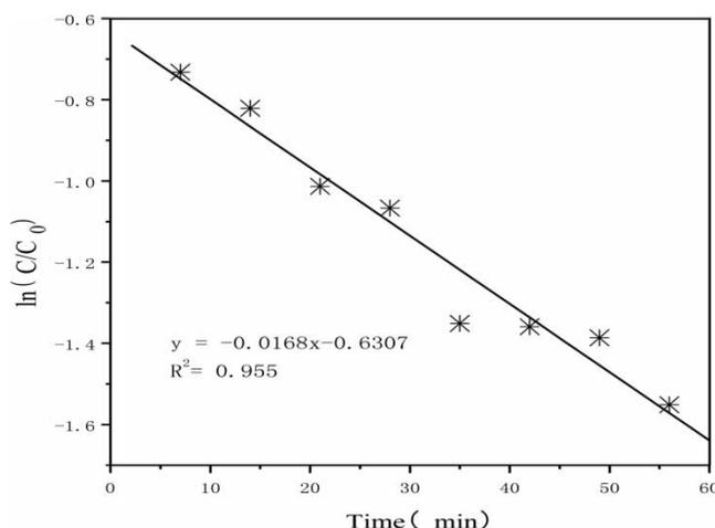
**Figure 6** | Pseudo-first-order kinetic model for Cr(VI) removal by M-NZVI. The M-NZVI particles have a (MCM-41):Fe<sup>0</sup> mass ratio of 4:1. [Cr(VI)]<sub>0</sub> = 100 mg/L, [M-NZVI]<sub>0</sub> = 1.0 g/L, and [pH]<sub>0</sub> = 6.0.
