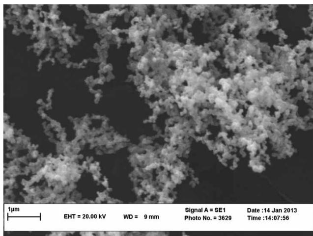
Figure 4 | SEM image of NiFe<sub>2</sub>O<sub>4</sub> nanoparticles.
