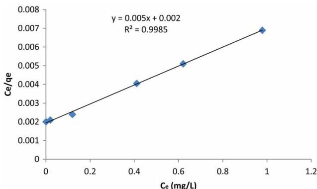
**Figure 9** | The Langmuir adsorption isotherm of NiFe<sub>2</sub>O<sub>4</sub> magnetic nanoparticles (0.05 g) for Cu(II) ions.
