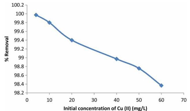
**Figure 8** | Effect of initial Cu(II) concentration on the removal of Cu(II) (adsorbent dose = 0.05 g, pH = 6, contact time = 25 min, and  $T = 298$  K).
