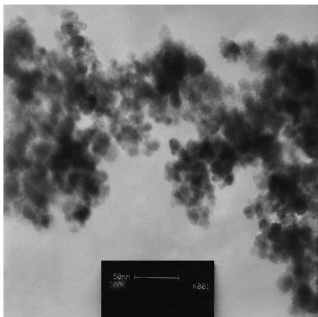
Figure 3 | TEM image of NiFe<sub>2</sub>O<sub>4</sub> nanoparticles.
