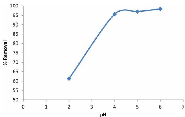
Figure 5 | Percentage of copper removal at different pH values (initial Cu(II) concentration = 4 mg/L, adsorbent dose = 0.05 g, and  $T = 298$  K).
