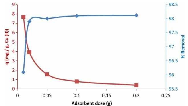
**Figure 7** | The effect of adsorbent dosage on the removal percentage of Cu(II) ions (initial Cu(II) concentration = 4 mg/L, pH = 6, contact time = 25 min, and  $T = 298$  K).
