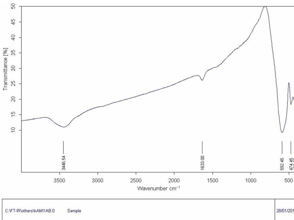
**Figure 1** | The FT-IR spectrum of NiFe<sub>2</sub>O<sub>4</sub> nanoparticles.
