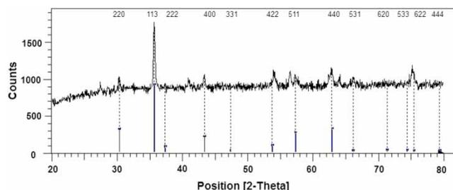
Figure 2 | XRD pattern of NiFe<sub>2</sub>O<sub>4</sub> nanoparticles.
