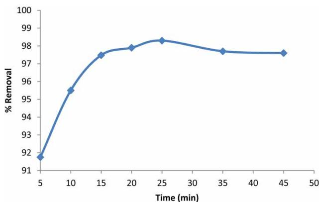
**Figure 6** | Effect of contact time (initial Cu(II) concentration = 4 mg/L, adsorbent dose = 0.05 g, pH = 6, and  $T = 298$  K).
