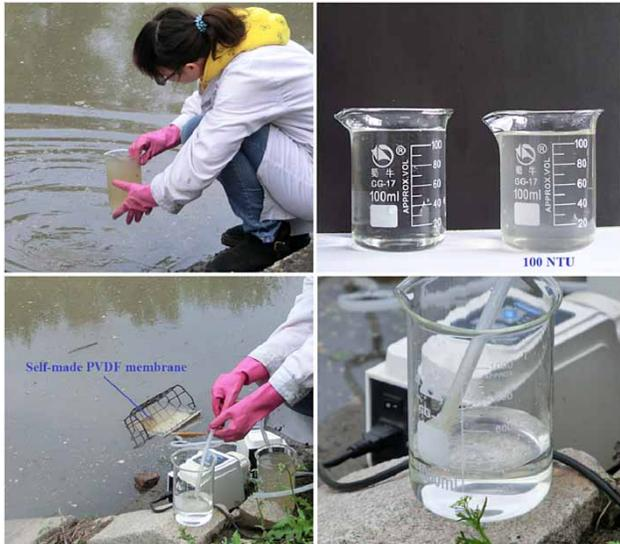
**Figure 3** | Change in the appearance of river water before and after treatment with a self-made pure PVDF membrane.
