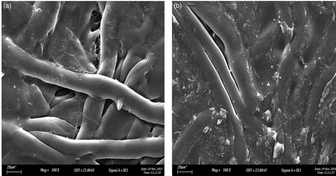
Figure 6 | SEM images for fouled (a) PVDF and (b) CA membranes (at a concentration 77 ppm).
