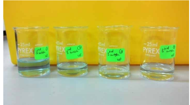
Figure 21 | Wastewater color changes for 22 ppm CA membrane after filtration.
