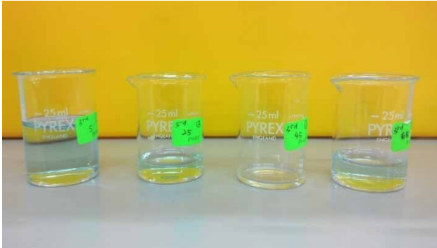
Figure 18 | Wastewater color changes for 22 ppm PVDF membrane after filtration.
