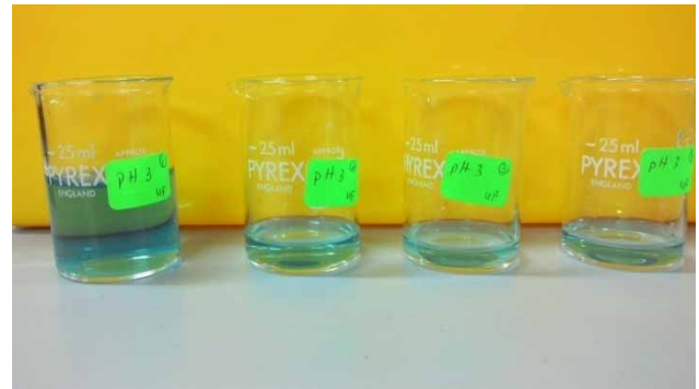
Figure 23 | Wastewater color changes for pH 3 CA membrane after filtration.
