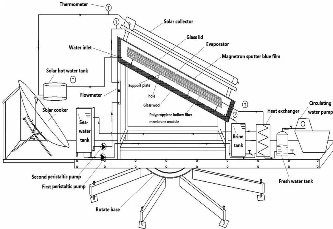
Figure 1 | Schematic diagram of test system.
