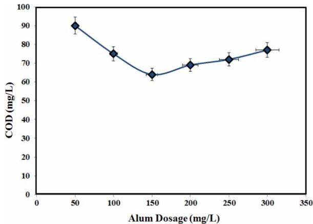
**Figure 7** | Effect of alum dosage on final COD for biodiesel wastewater.
