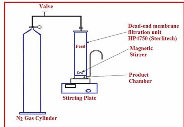
**Figure 1** | Schematic diagram of the dead-end test rig for flux decline test.
