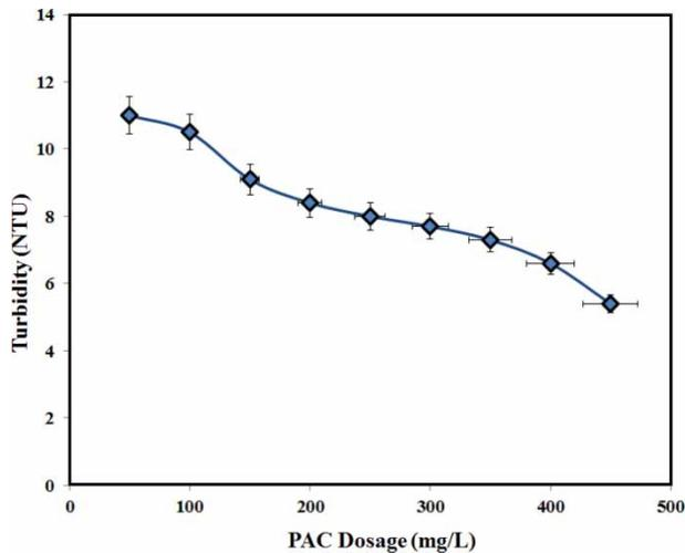
Figure 5 | Effect of different PAC dosages on turbidity removal.
