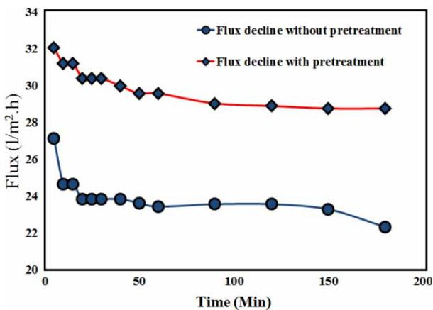
**Figure 8** | Comparison between flux decline with and without pretreatment for the second sample.
