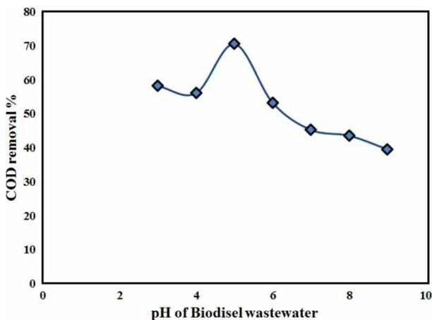
Figure 6 | Effect of pH on COD removal at 400 mg/L PAC.
