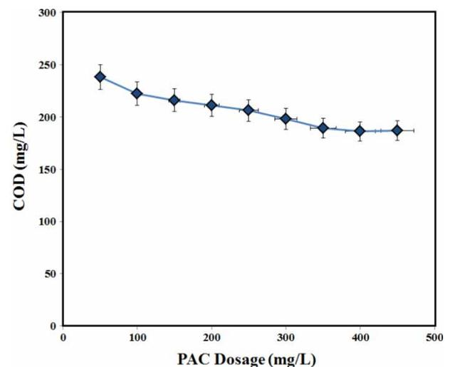
**Figure 4** | Effect of different PAC dosages on COD removal.
