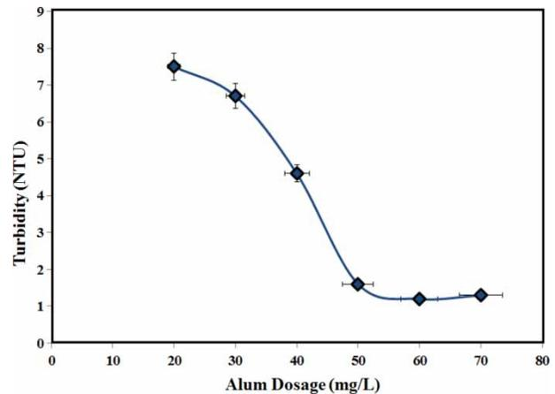
Figure 2 | Effect of alum dosage on final turbidity for treated effluent wastewater.
