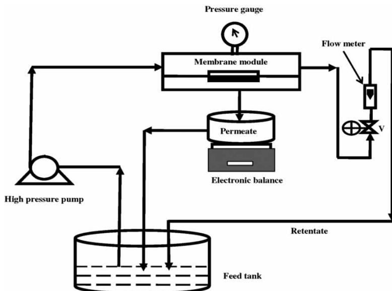
Figure 1 | Schematic of cross-flow ultrafiltration setup (V = retentate valve).
