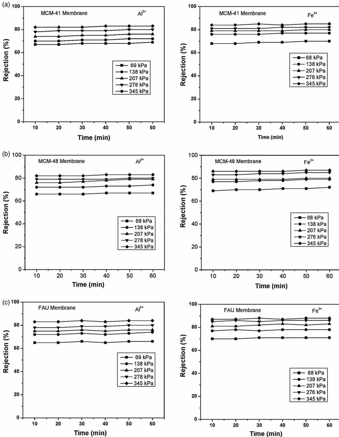
**Figure 7** | Variation of rejection of  $Al^{3+}$  and  $Fe^{3+}$  with time at different applied pressures for (a) MCM-41, (b) MCM-48 and (c) FAU membranes (feed concentration = 250 ppm, pH = 2).
