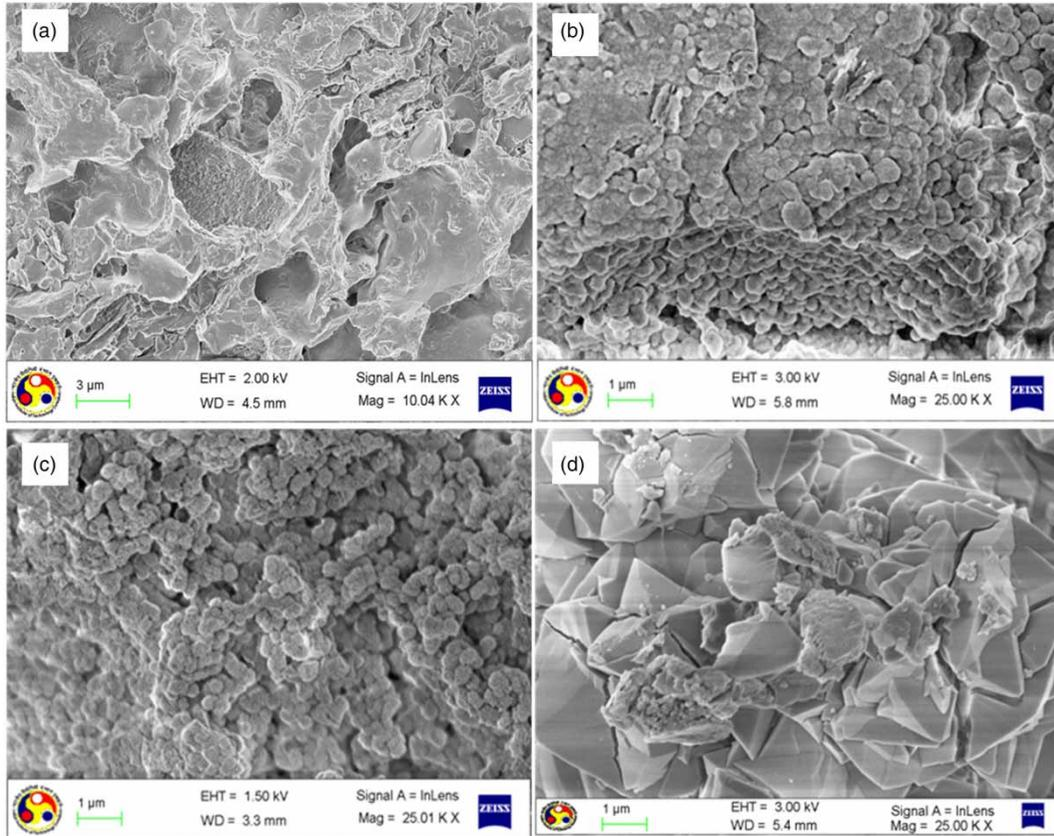
**Figure 3** | FESEM images of (a) ceramic support, (b) MCM-41, (c) MCM-48 and (d) FAU zeolite membranes.
