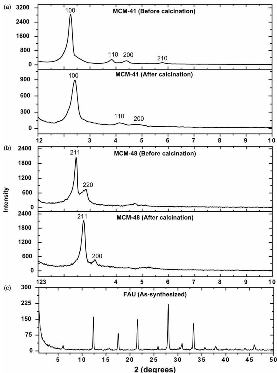
**Figure 2** | XRD patterns of (a) MCM-41 (before and after calcination), (b) MCM-48 (before and after calcination), and (c) FAU zeolite (as-synthesized) powder samples.
