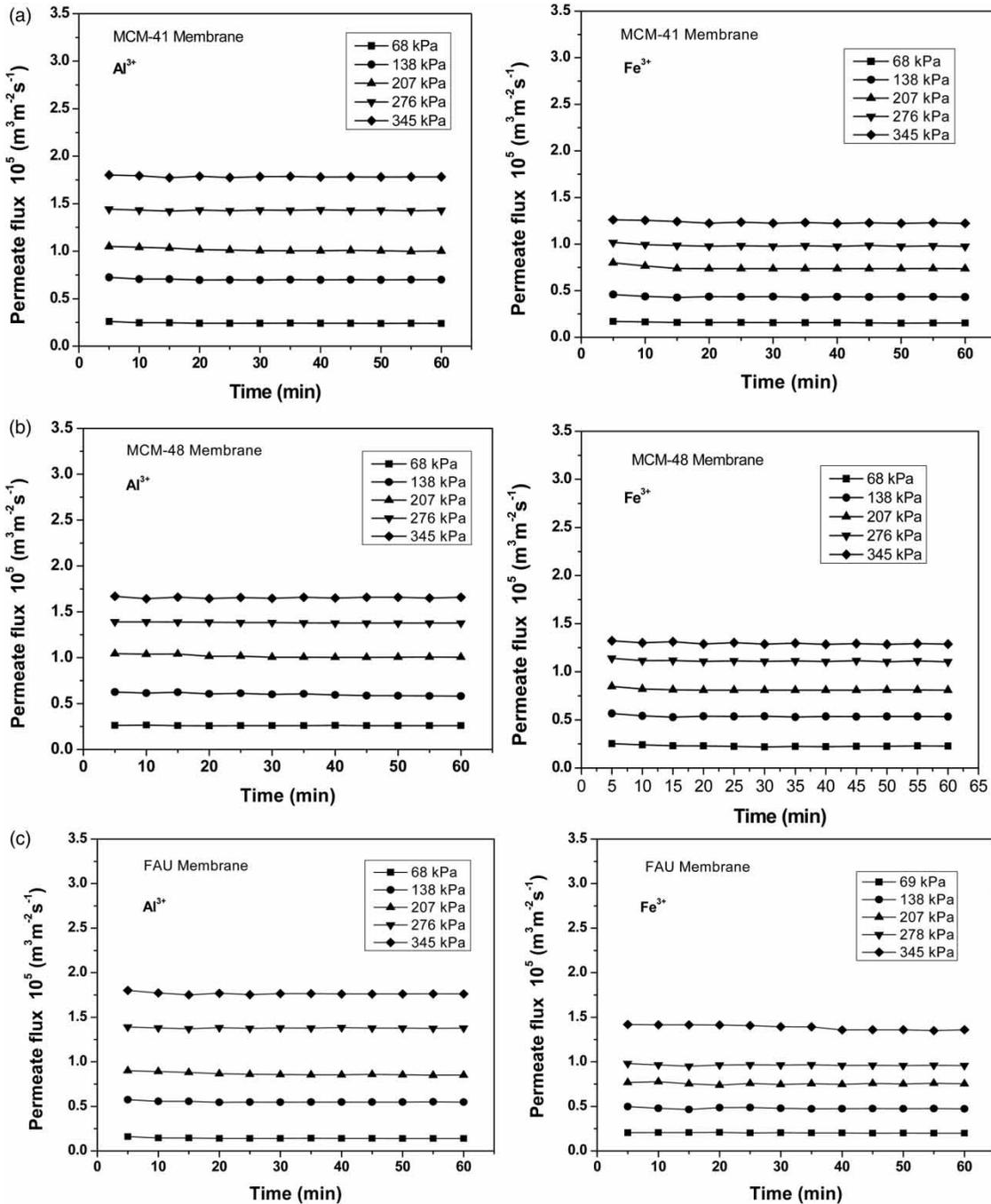
**Figure 6** | Variation of permeate flux of  $\text{Al}^{3+}$  and  $\text{Fe}^{3+}$  with time at different applied pressures for (a) MCM-41, (b) MCM-48 and (c) FAU membranes (feed concentration = 250 ppm, pH = 2).
