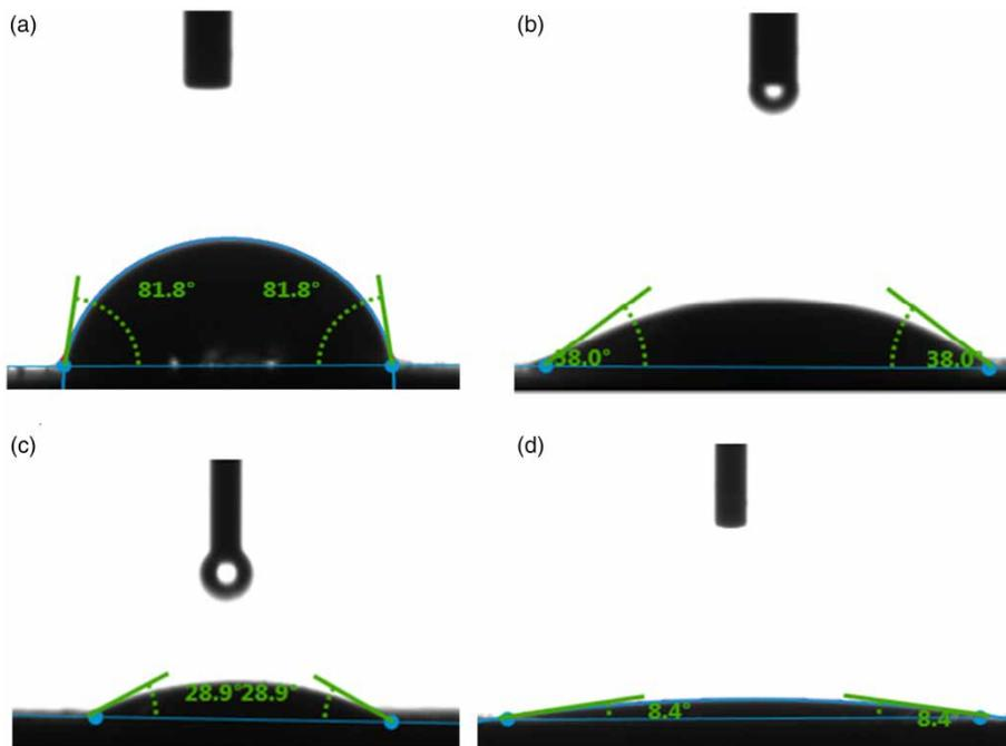
**Figure 4** | Contact angles of (a) support, (b) MCM-41, (c) MCM-48 and (d) FAU zeolite membranes.
