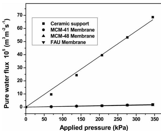
Figure 5 | Pure water flux as a function of applied pressure for support and zeolite membranes.
