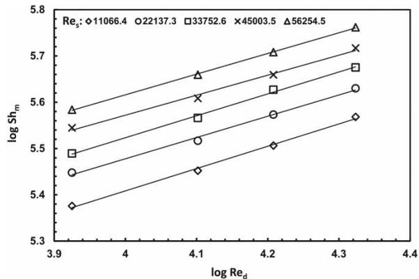
**Figure 9** | Effect of  $Re_d$  on  $Sh_m$  at different  $Re_s$  (concentration of copper sulphate = 0.02 M, concentration of naphthenic acid = 0.1 M, continuous phase flow rate = 200 cm<sup>3</sup>/s, degree of roughness = 1 mm).
