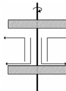
Figure 6 | Flow pattern at two parallel rotating discs.
