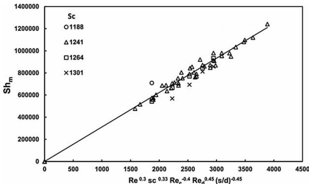
**Figure 11** | Overall mass correlation at a rotating rough disc.
