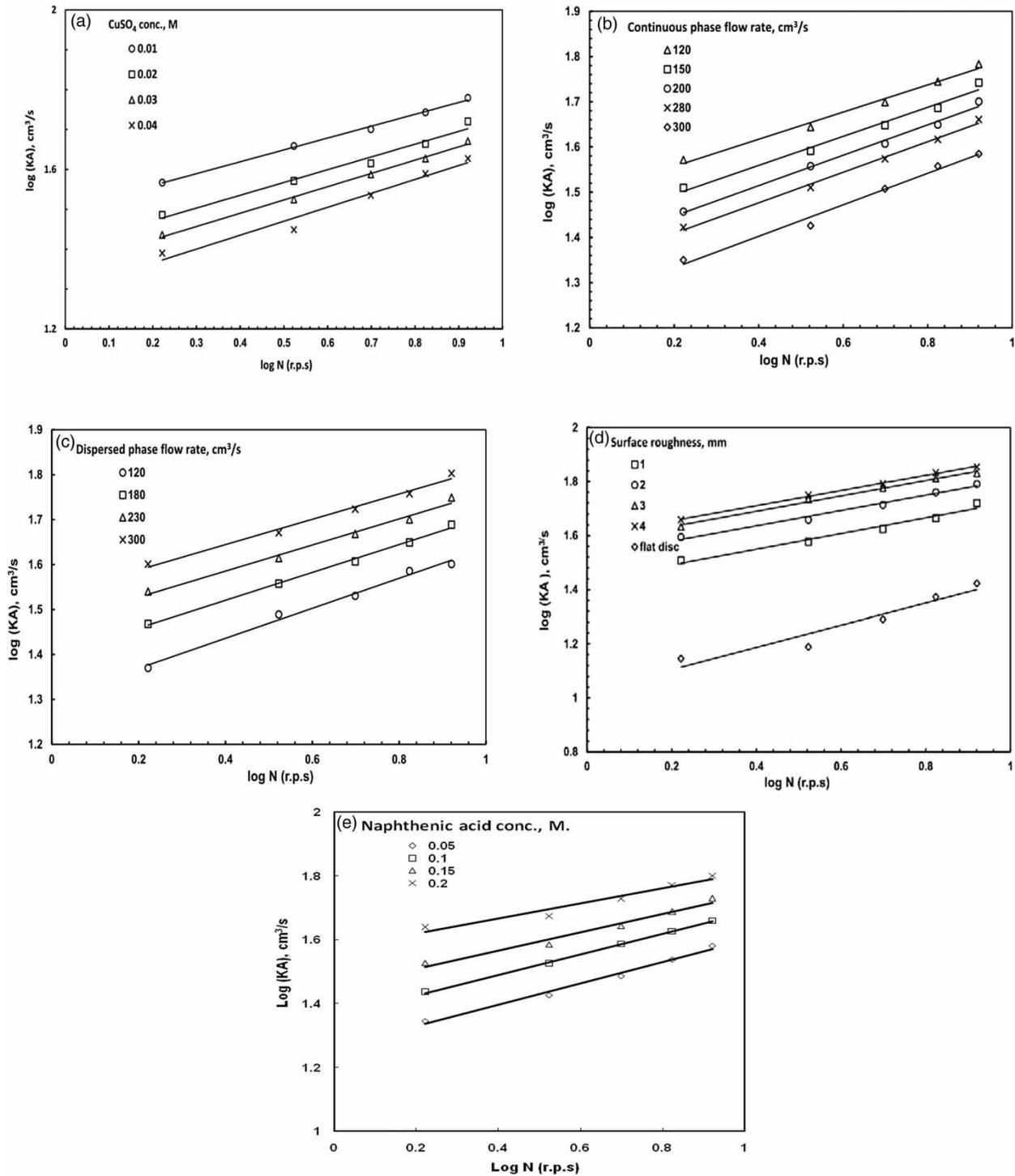
**Figure 4** | Effect of rotational speed on the volumetric mass transfer coefficient ((a) at different initial  $\text{CuSO}_4$  concentrations, (b) at different continuous phase flow rate,  $\text{cm}^3/\text{s}$ , (c) at different dispersed phase flow rate, (d) at different degree of roughness, (e) at different concentration of naphthenic acid).
