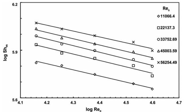
**Figure 8** | Effect of  $Re_c$  on  $Sh_m$  at different  $Re_s$  (concentration of  $CuSO_4 = 0.01$  M, concentration of naphthenic acid = 0.1 M, dispersed phase flow rate = 180 cm<sup>3</sup>/s, degree of roughness = 1 mm).
