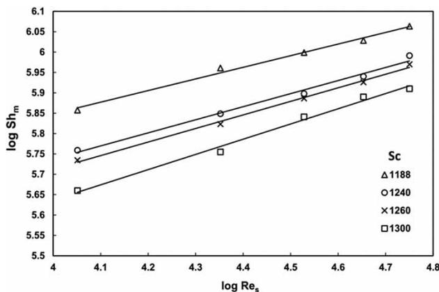
**Figure 7** | Effect of  $Re_s$  on  $Sh_m$  at different  $Sc$  (continuous phase flow rate = 200 cm<sup>3</sup>/s, dispersed phase flow rate = 180 cm<sup>3</sup>/s, naphthenic acid concentration = 0.1 M, degree of roughness = 1 mm).
