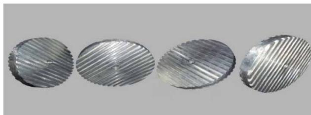
Figure 2 | Grooved disc with different degree of roughness.
