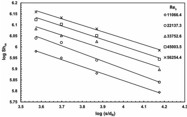
**Figure 10** | Effect of the dimensionless ratio ( $S/d_R$ ) disc geometry on  $Sh_m$  (concentration of copper sulphate = 0.02 M, concentration of naphthenic acid = 0.1 M, continuous phase flow rate = 200 cm<sup>3</sup>/s, dispersed phase flow rate = 180 cm<sup>3</sup>/s).
