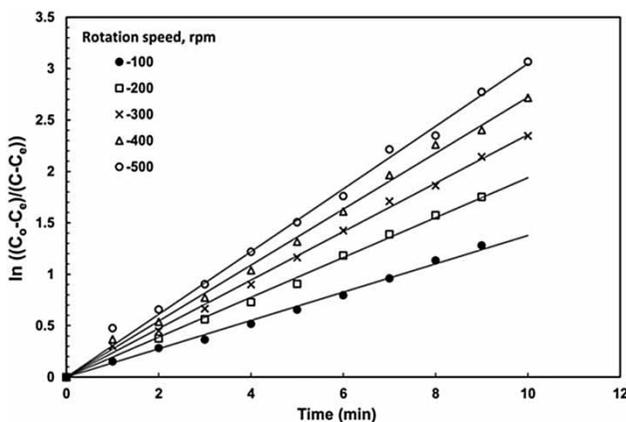
**Figure 3** | Typical plots of concentration-time at different rotational speed ( $\text{CuSO}_4$  conc. = 0.01 M, naphthenic acid conc. = 0.1 M, continuous phase flow rate =  $200 \text{ cm}^3/\text{sec}$ , dispersed phase flow rate =  $180 \text{ cm}^3/\text{sec}$ , degree of roughness = 1 mm).
