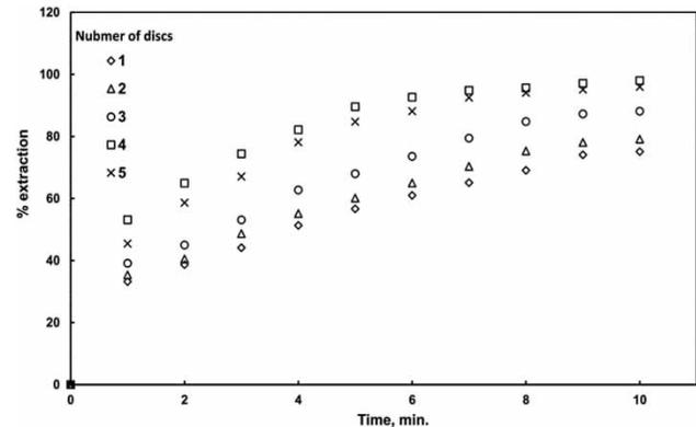
Figure 5 | Effect of number of discs on % extraction ( $\text{CuSO}_4$  conc. = 0.01 M; Naphthenic acid conc. = 0.1 M; rotation speed = 500 rpm; Continuous phase flow rate =  $200 \text{ cm}^3/\text{s}$ ; Dispersed phase flow rate =  $180 \text{ cm}^3/\text{s}$ ; degree of roughness = 2 mm).
